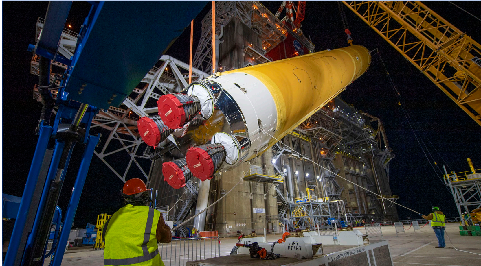
Crews at Stennis Space Center worked Jan. 21-22 to install the first flight core stage of NASA's new Space Launch System in the B-2 Test Stand for a series of Green Run tests in coming months. Operations required crews to lift the massive core stage from a horizontal position into a vertical orientation, a procedure known as "break over." Once the stage was oriented in a horizontal position on the night of Jan. 21, crews tied it in place to await favorable win conditions. The following morning, a beautiful south Mississippi sunrise framed the core stage (page 5 photo) as crews began the process of raising, positioning and securing the stage on the stand. The upcoming Green Run series represents the first top-to-bottom integrated testing of the stage's systems prior to its maiden Artemis I test flight.
