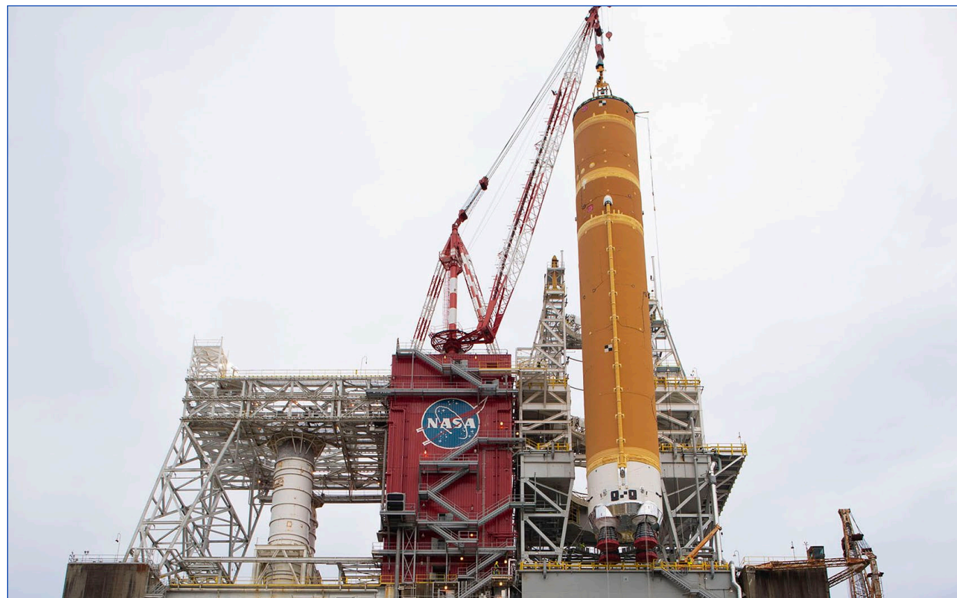
Crews at Stennis Space Center worked Jan. 21-22 to install the first flight core stage of NASA's new Space Launch System in the B-2 Test Stand for a series of Green Run tests in coming months. Operations required crews to lift the massive core stage from a horizontal position into a vertical orientation, a procedure known as "break over." Once the stage was oriented in a horizontal position on the night of Jan. 21, crews tied it in place to await favorable win conditions. The following morning, a beautiful south Mississippi sunrise framed the core stage (page 5 photo) as crews began the process of raising, positioning and securing the stage on the stand. The upcoming Green Run series represents the first top-to-bottom integrated testing of the stage's systems prior to its maiden Artemis I test flight.
