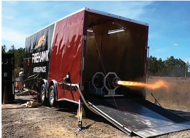
Firehawk Aerospace uses a newly built "roadable test stand" to conduct hot fire testing of its Armstrong 1k test article Dec. 1, 2021, at Stennis. The small start-up company is seeking to revolutionize hybrid rocket engine technology with its patented 3-D printed solid fuel. (Firehawk Aerospace)
