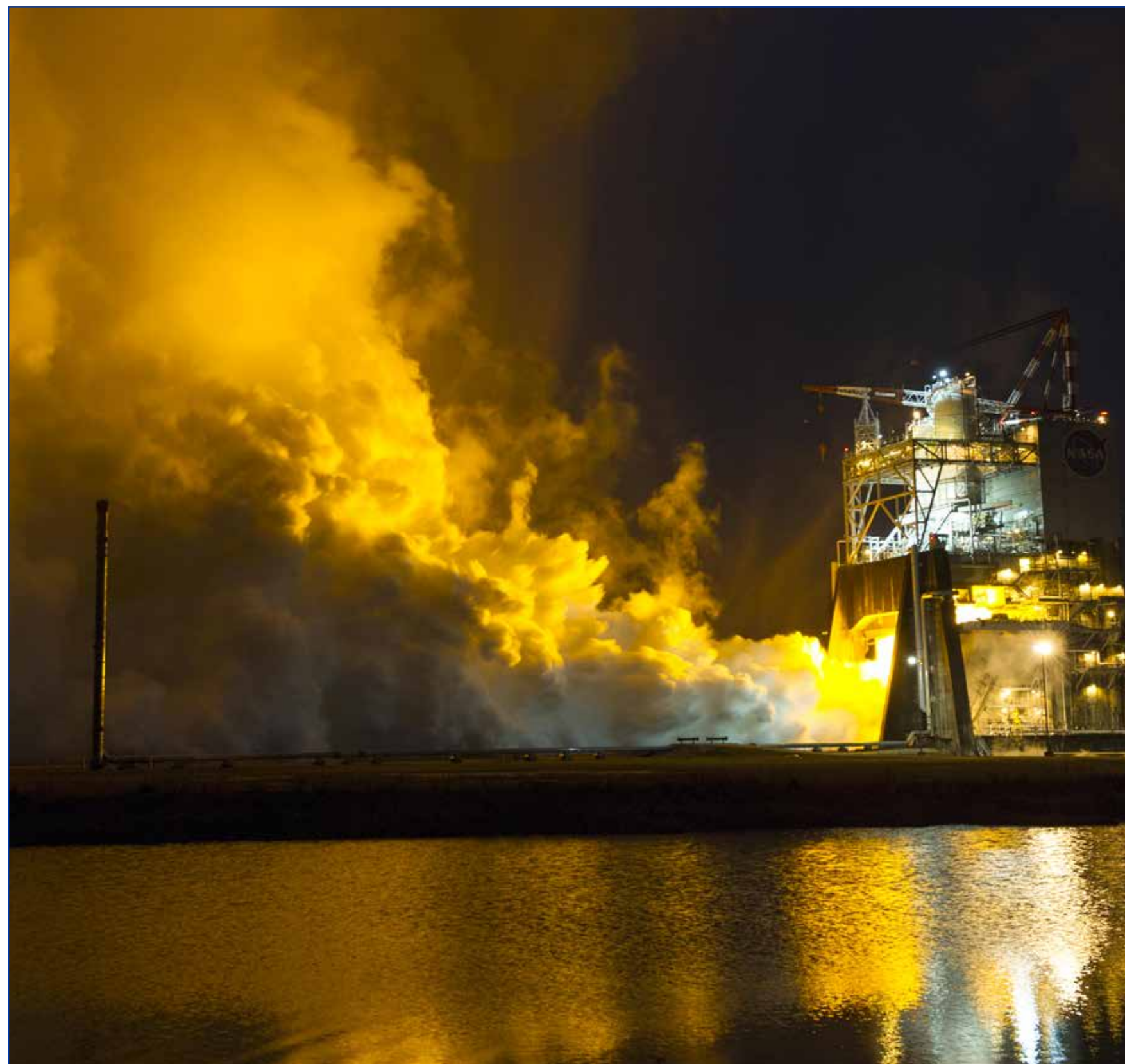
NASA conducts the first of a series of developmental tests on the RS-25 rocket engine on the A-1 Test Stand at Stennis Space Center on January 9, 2015.
