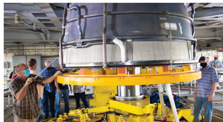
Technicians on the engine deck of the Fred Haise Test Stand at Stennis prepare to use a vertical engine installer (VEI) to support, detach, and lower the nozzle from RS-25 development engine No. 0528 (bottom left). Once lowered the technicians examine the detached nozzle (top) and ensure all is in place (bottom right) during an RS-25 rocket engine nozzle remove-and-replace procedure Oct. 13.
