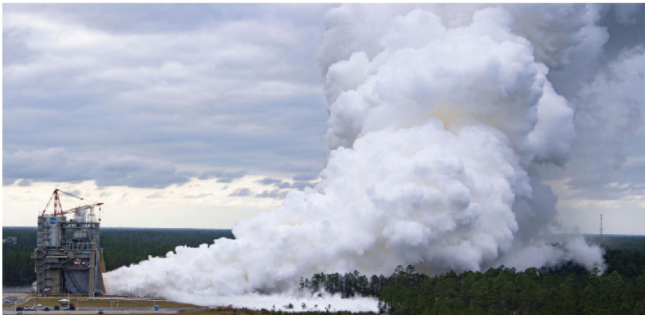
NASA conducts a full-duration (500 seconds) hot fire test of RS-25 developmental engine No. 0525 on the Fred Haise Test Stand at Stennis Space Center on Dec. 15. The hot fire marked the first in a new series of tests to collect performance data for production of RS-25 engines to help power NASA's Space Launch System rocket on future deep space missions.
