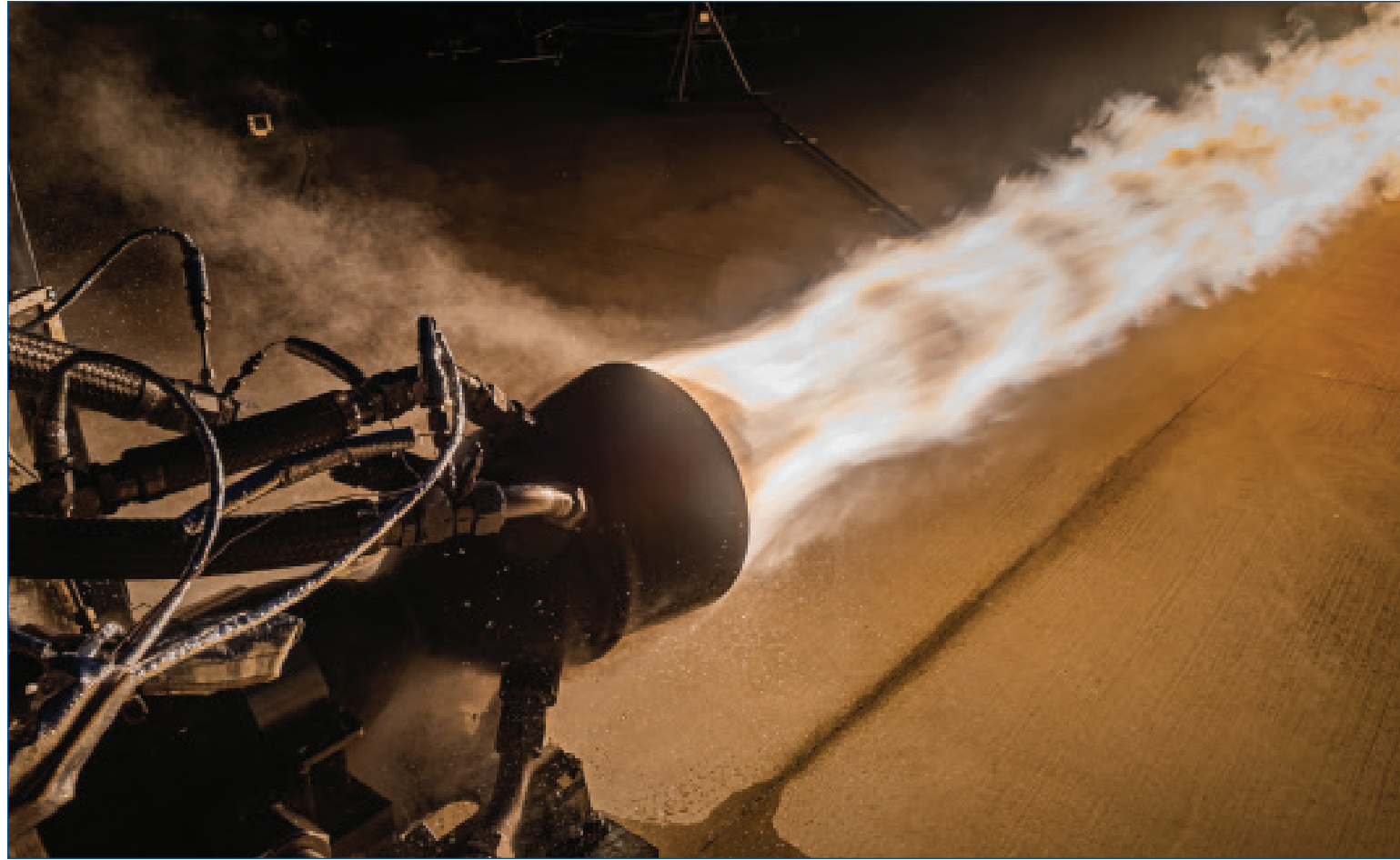
(Top left photo) Launcher's 3D-printed Engine-2 (E-2) rocket engine completes a 5-second hot fire Aug. 20 of its latest thrust chamber assembly (Credit: Launcher / John Kraus Photography). (Right photo) The arrival of two trusses marks the first of several large elements needed to prepare the B-2 Test Stand for Green Run testing of the Exploration Upper Stage unit being built for use on future Space Launch System missions. (Bottom left photo) The spike diffuser is a new design developed and tested at Stennis on the E-3 Test Stand.
