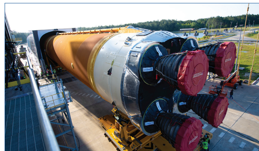
(Above photo) Crews at NASA's Stennis Space Center worked April 19-20 to remove the first flight core stage of the agency's Space Launch System (SLS) rocket from the B-2 Test Stand in preparation for its transport to Kennedy Space Center in Florida, following completion of the Green Run series of tests of its design and systems. The core stage was then oriented horizontally (bottom left photo) and loaded for departure from Stennis Space Center on April 21-22 (bottom center photo).
