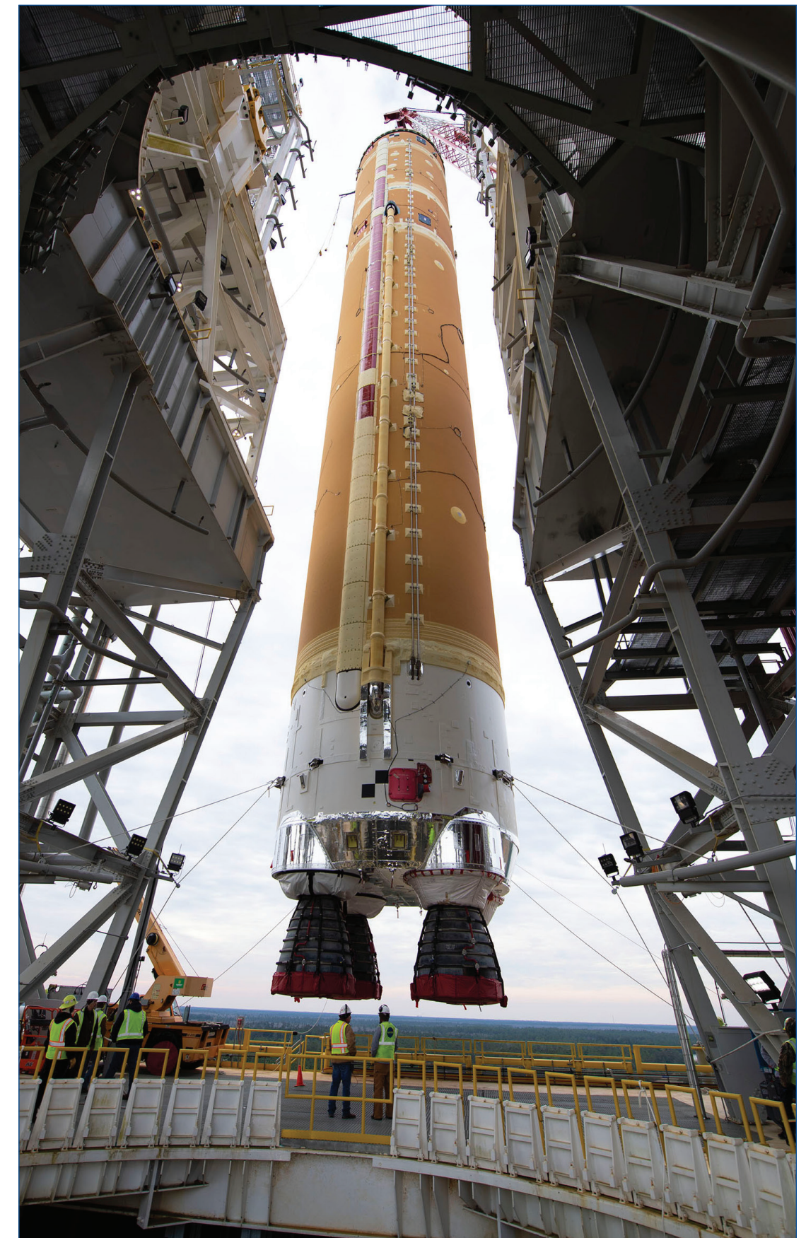
(Above photo) Crews at NASA's Stennis Space Center worked April 19-20 to remove the first flight core stage of the agency's Space Launch System (SLS) rocket from the B-2 Test Stand in preparation for its transport to Kennedy Space Center in Florida, following completion of the Green Run series of tests of its design and systems. The core stage was then oriented horizontally (bottom left photo) and loaded for departure from Stennis Space Center on April 21-22 (bottom center photo).
