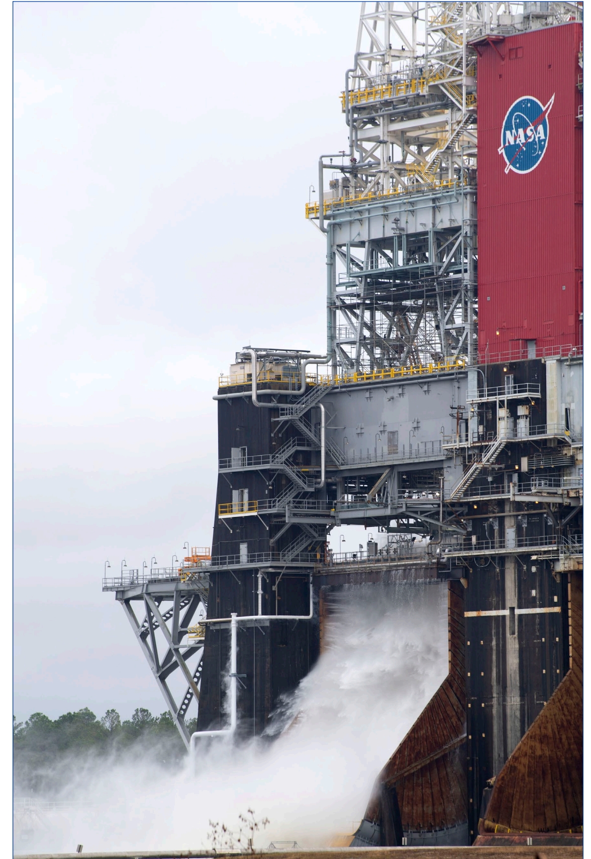
(Right photo) Water flows into the B-2 Test Stand flame deflector Dec. 13 during a simulated Space Launch System core stage test.
