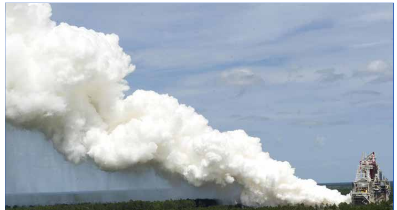
(Top photo) NASA conducts a successful 500-second test of the first RS-25 flight engine on the A-1 Test Stand at Stennis Space Center. The next time engine No. 2059 fires for that length of time, it will be carrying astronauts on their first deep-space mission in more than 45 years.
