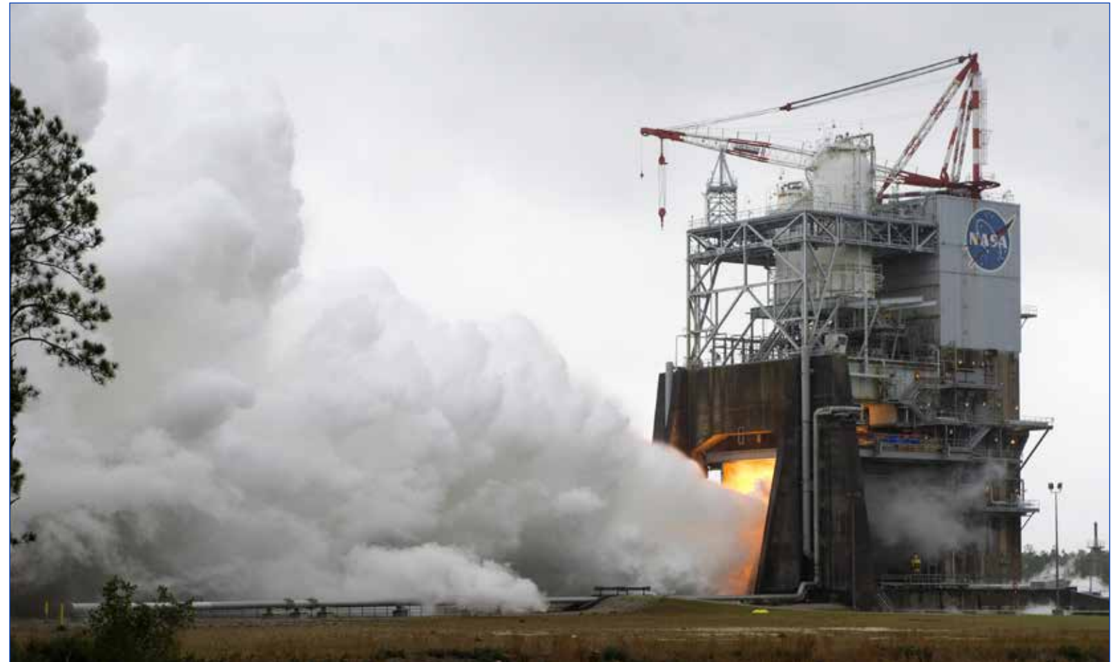
(Top photo) NASA conducts a successful 500-second test of the first RS-25 flight engine on the A-1 Test Stand at Stennis Space Center. The next time engine No. 2059 fires for that length of time, it will be carrying astronauts on their first deep-space mission in more than 45 years.
