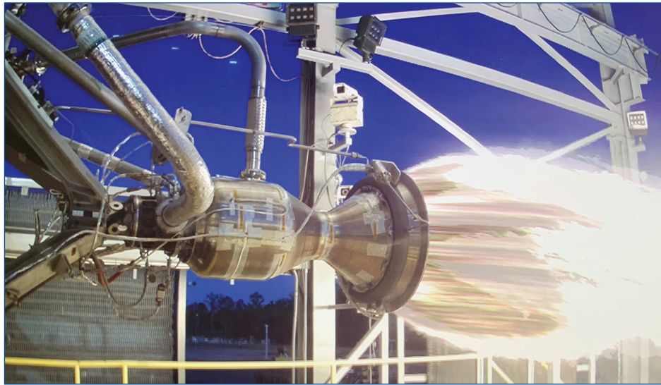
Virgin Orbit, a satellite-launch company, partnered with Stennis Space Center to successfully test their Thrust Chamber Assembly, running a hot fire test campaign for a total of 974.391 seconds.
