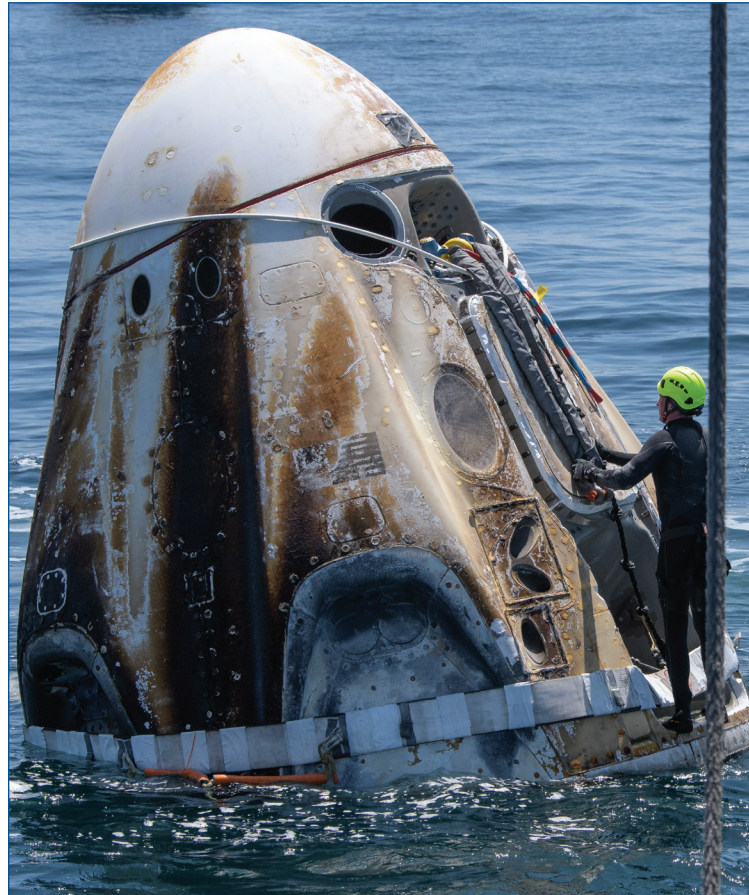
(Left photo) A support team member examines the SpaceX Crew Dragon Endeavour spacecraft shortly after it landed in the Gulf of Mexico off the coast of Pensacola, Florida, on Aug. 2. The Demo-2 test flight was the first to deliver astronauts to the International Space Station and return them safely to Earth onboard a commercially built and operated spacecraft.
