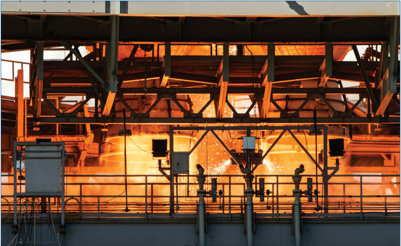
(Above photo) A telephoto view offers a look at the four RS-25 engines firing during the Space Launch System core stage hot fire March 18.
