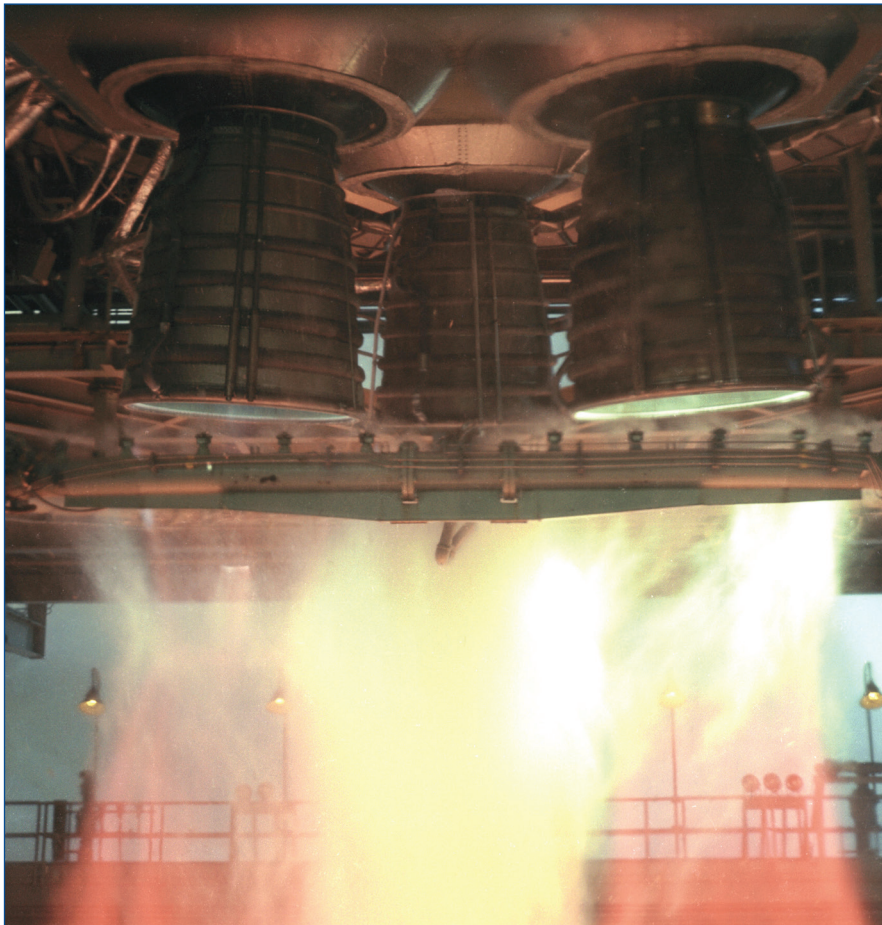
A trio of space shuttle main engines fire simultaneously during a test of the vehicle main propulsion test article on the B-2 Test Stand at Stennis. The series of tests to certify the design and operation of the shuttle propulsion system was a critical milestone leading up to the maiden launch of the vehicle and is considered by many to represent one of Stennis' finest hours.
