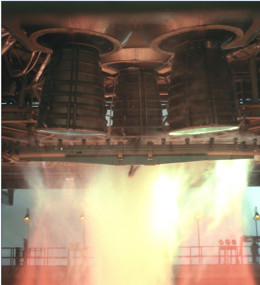
A trio of space shuttle main engines fire simultaneously during a test of the vehicle main propulsion test article on the B-2 Test Stand at Stennis. The series of test to certify the design and operation of the shuttle propulsion system was a critical milestone leading up to the maiden launch of the vehicle and is considered by many to represent one of Stennis' finest hours.
