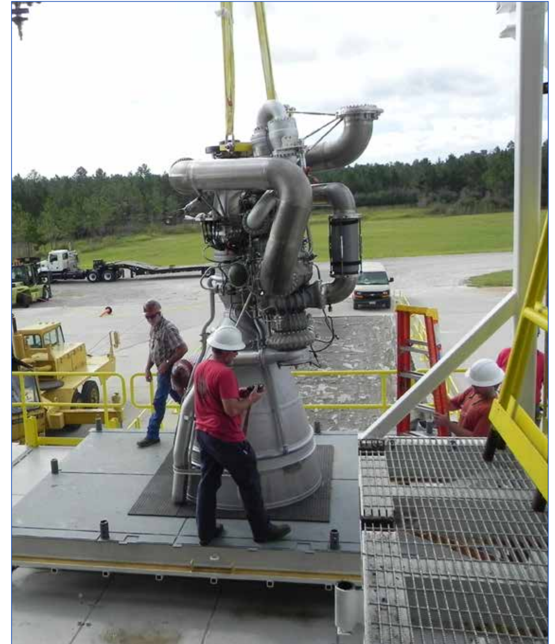
(Right photo) E-1 Test Stand team members help move an Aerojet Rocketdyne AJ26 engine into place on the stand. Acceptance testing of AJ26 engines to power Orbital Sciences Corporation flights will resume in late October.
