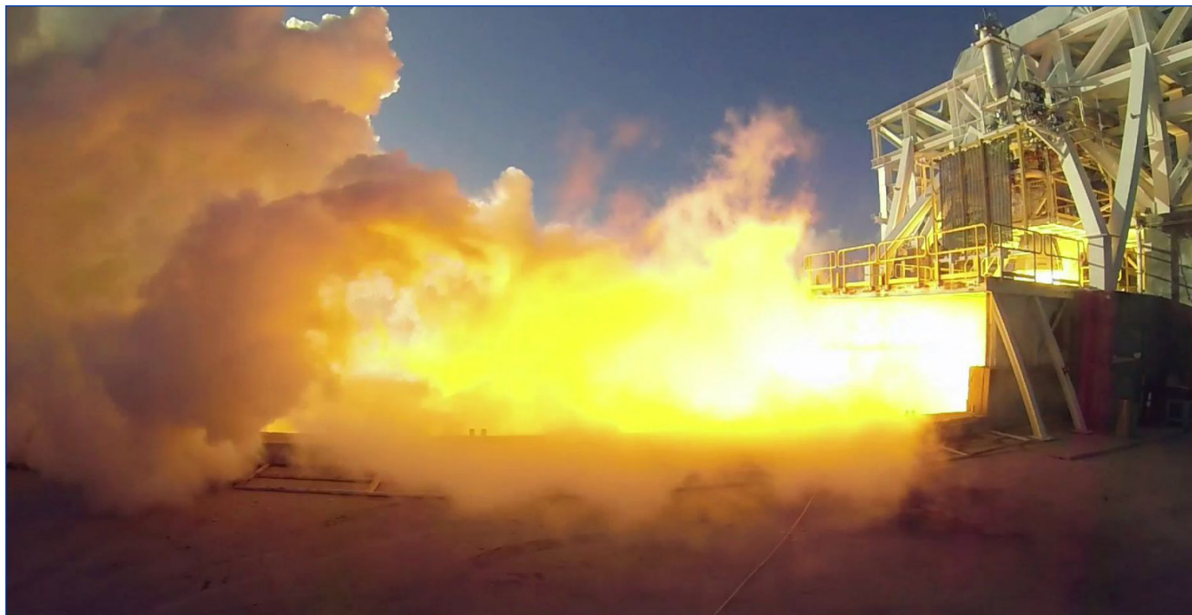
A team of NASA, Orbital Sciences Corporation, Aerojet Rocketdyne and Lockheed Martin engineers conduct a hotfire test of Aerojet Rocketdyne AJ26 engine E-15 on the E-1 Test Stand at NASA's Stennis Space Center on Jan. 17.
