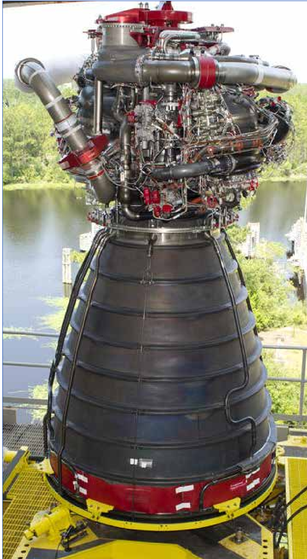
(Left photo) RS-25 rocket engine No. 0525 sits on the deck of the A-1 Test Stand on July 17 in preparation for installation and a series of hotfire tests.
