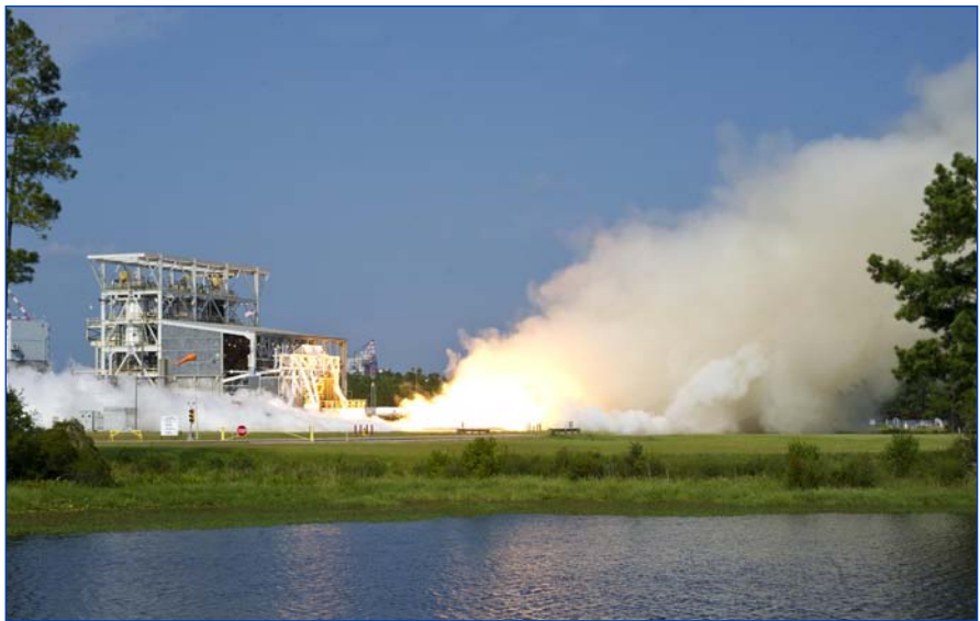
NASA, Orbital Sciences Corporation and Aerojet Rocketdyne engineers conduct a full-duration test of an AJ26 engine on the E-1 Test Stand at Stennis Space Center on Aug. 8.
