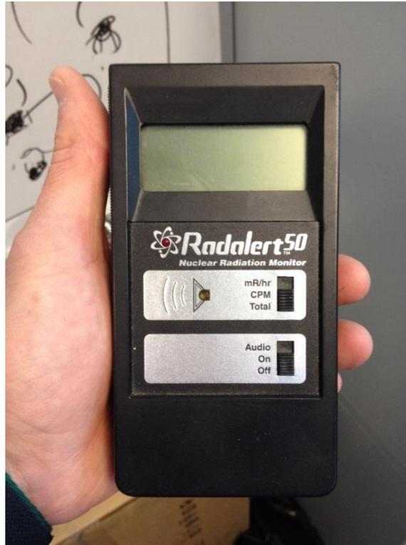
**Figure 44 - Radalert50 Nuclear Radiation Monitor**
