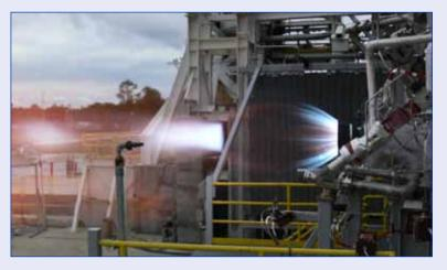
Blue Origin successfully test fires its BE-3 high-performance liquid hydrogen engine thrust chamber at NASA's Stennis Space Center. (Image credit: Blue Origin)
