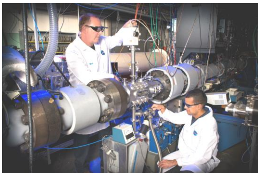
Electric Arc Shock Tube Outer Planetary Entry & Radiation / Ionization Study
