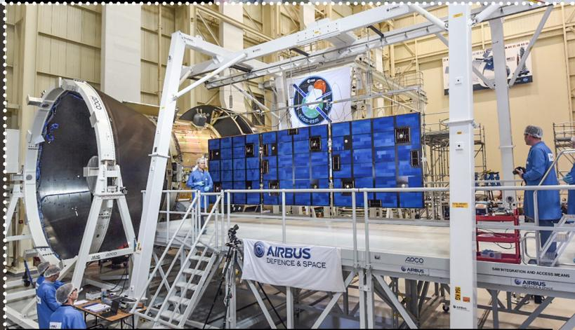
**Service Module Structural Testing**
