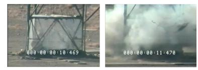
(Far left) Test cell candle initiation in 8' x 8' test cell with Lexan flexible sheets
