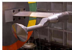
MSL model in LaRC 31-Inch Mach 10 Wind Tunnel.
