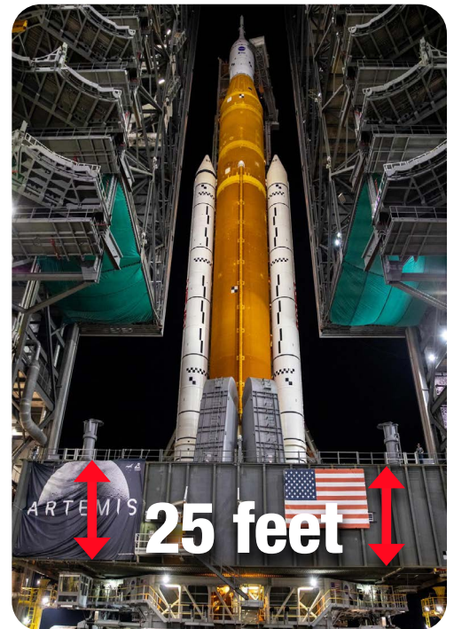
The Mobile Launcher (ML) at Kennedy Space Center was originally constructed for transporting the Saturn V rocket. The base alone is 25-feet high.
