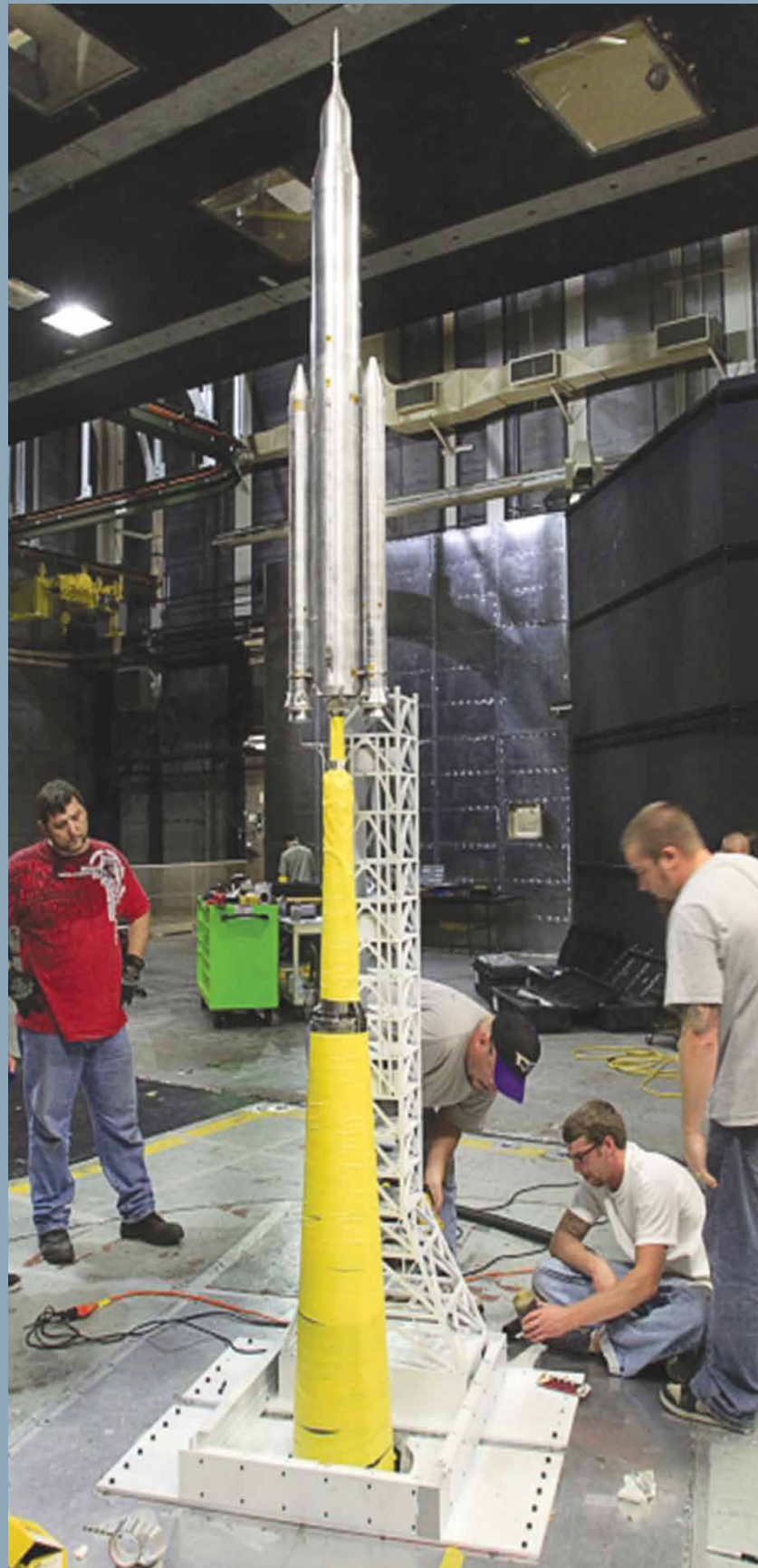
NASA engineers and technicians tested four payload configurations during the liftoff transition testing of a 67.5-inch model of the SLS in Langley's 14-by-22-Foot Subsonic Tunnel.
