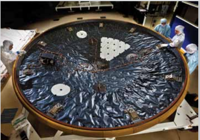
The heat shield for the Mars Science Laboratory launched in November carried a set of sensors developed with Langley's help.
