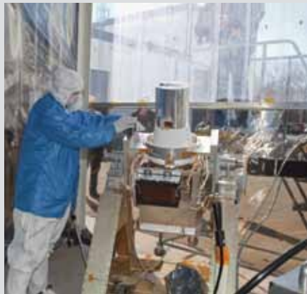
Checkout of the SAGE III-ISS instrument, which is planned for launch in 2014. SAGE stands for Stratospheric Aerosol and Gas Experiment.
