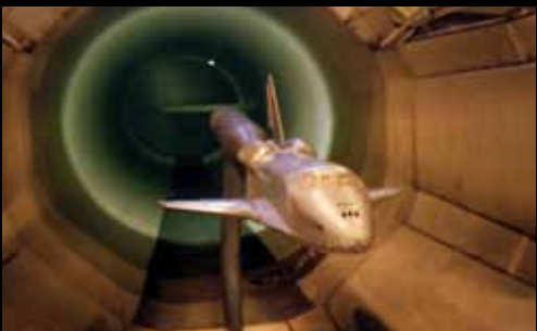
A scale model of the shuttle being tested in Langley's 16-Foot Transonic Tunnel.
