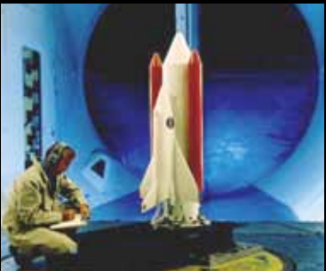
An early shuttle design undergoing tests in the Transonic Dynamics Tunnel in 1972.
