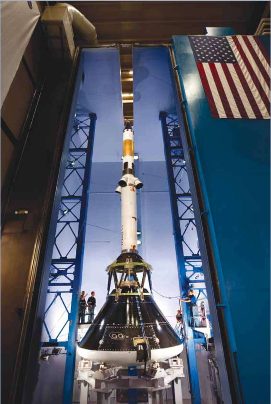
Crew capsule and launch abort system undergoing acoustic and vibration tests.
