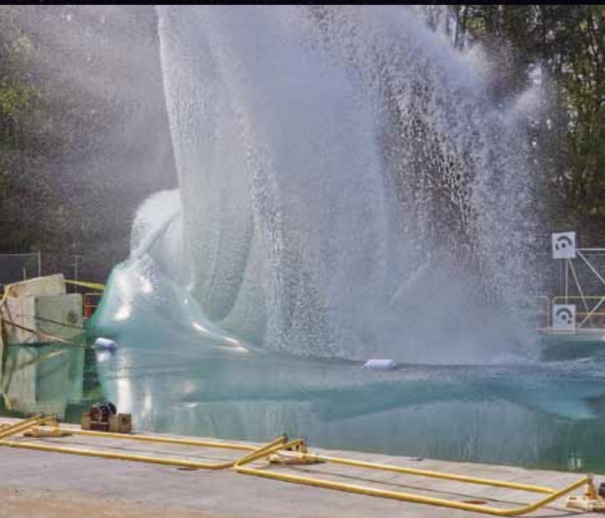
The Orion crew capsule mockup lands in the Hydro Impact Basin during a drop test at Langley.
