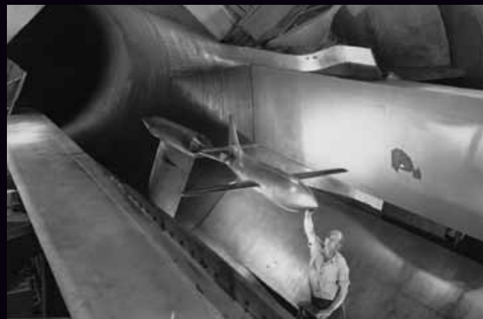
Bell X-1 model mounted in the slotted test section of the 16-Foot Tunnel, 1951.
