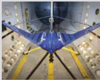
A joined wing model in the TDT.
