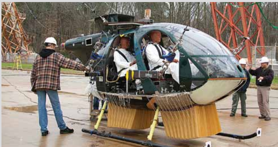
Researchers dropped a helicopter to see if a deployable energy absorber lessened the force of the crash.
