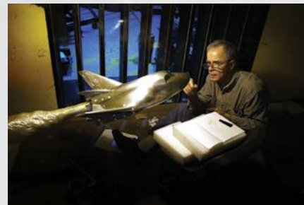
Above left: Researchers test a component of an inflatable device that could be used in future missions for spacecraft atmospheric re-entry. Center: Technician Rick Hall inside the Unitary Plan Wind Tunnel readying a Dream Chaser model for tests in support of NASA's Commercial Crew initiative. Above right: A mock-up to test concepts for capturing an asteroid.
