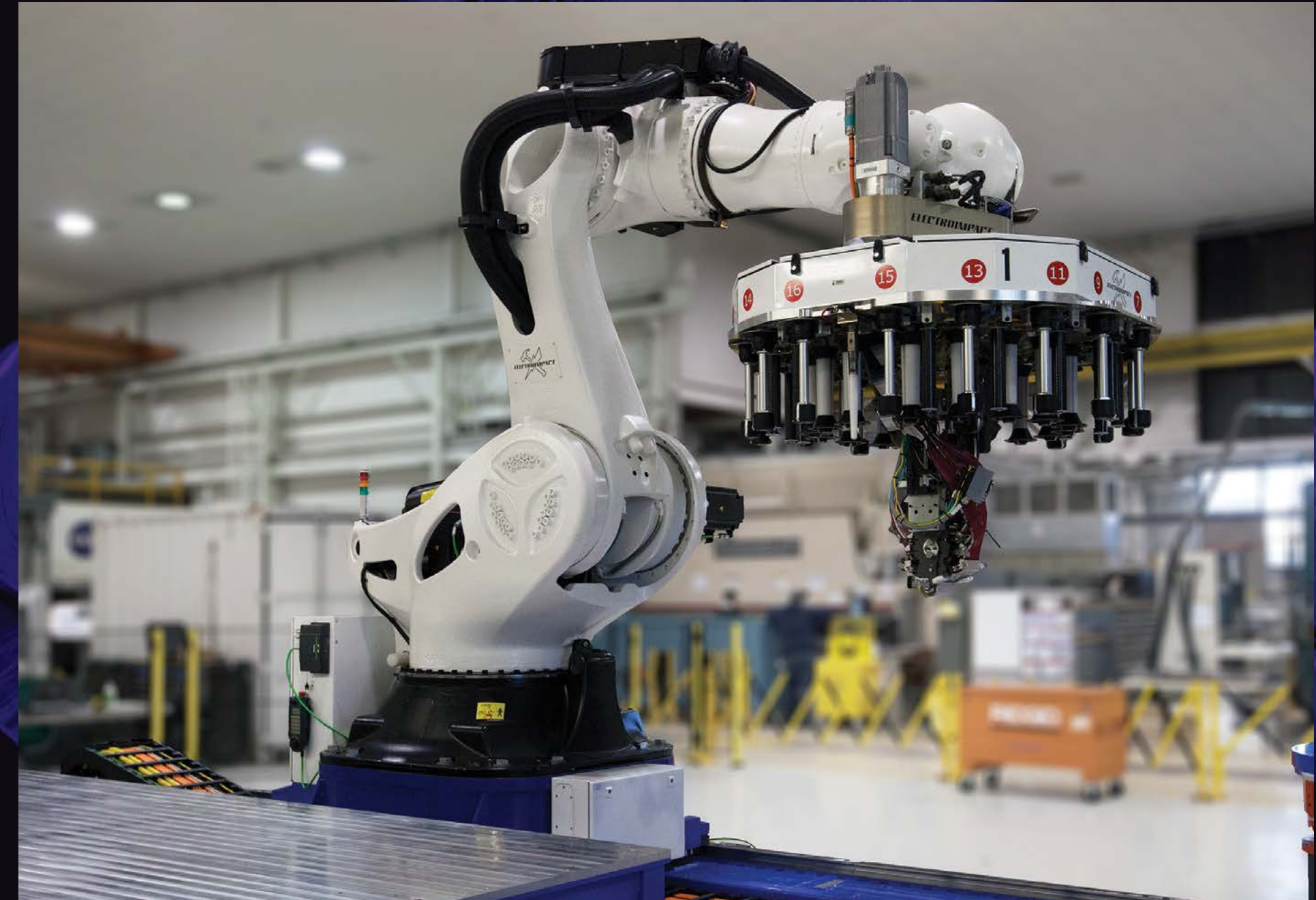
It looks like something out of a Transformers movie – a huge robotic arm that moves and spins to pick up massive heads filled with spools of carbon fibers, then moves in preprogrammed patterns to deposit those fibers onto a 40-foot bed. But instead of transforming from machine to Autobot, it can transform epoxy and fibers into aerospace structures and parts. Its name is ISAAC, or Integrated Structural Assembly of Advanced Composites.
