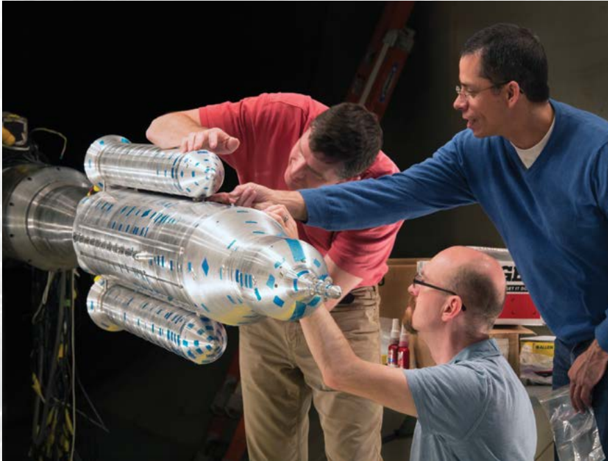
Above: The aerodynamics team at Langley tested a model of the 70-metric-ton Space Launch System—NASA's heavy-lift launch vehicle that will carry crew, cargo and science missions into deep space.
