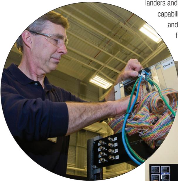
Marshall's Systems Integration Lab conducts HWIL testing to reduce SLS flight software development risk.
