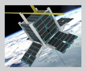
ChargerSat-1's mission is to conduct three technology demonstrations: a gravity gradient stabilization system will passively stabilize the spacecraft; deployable solar panels will nearly double the power input to the spacecraft; and the same deployable solar panels will shape the gain pattern of a nadir-facing monopole antenna, allowing improved horizon-to-horizon communications.
