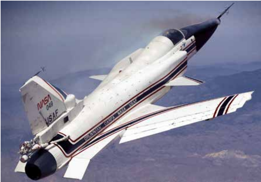
The second X-29A on a high-AoA research flight. Note the deflected canards, tufts (to reveal flow patterns), and smoke visualization employment. (NASA)
