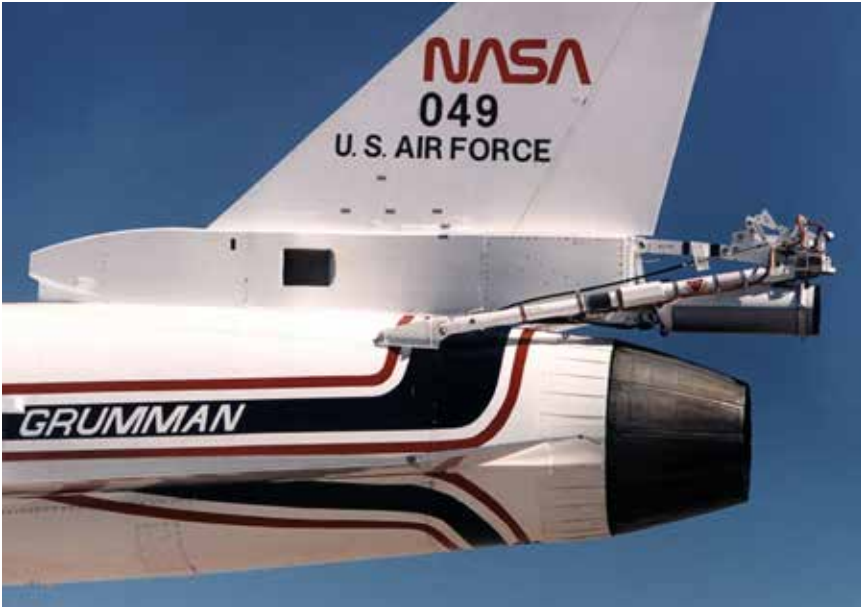
The spin-parachute installation on the second Grumman X-29 aircraft, 1989. Note as well the stylized and controversial “NASA worm” on the vertical fin, which was a source of annoyance for veteran NASA traditionalists. (NASA)
