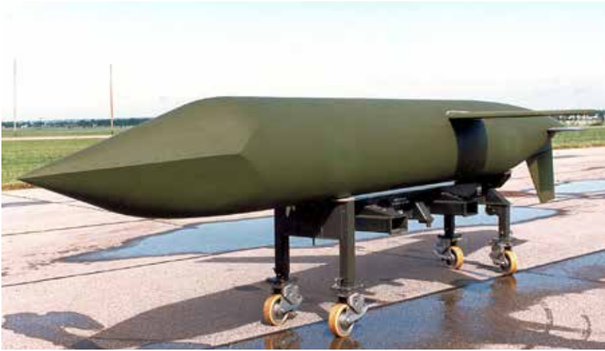
The General Dynamics AGM-129 Advanced Cruise Missile incorporated a small forward swept wing. (USAF via NASA)
