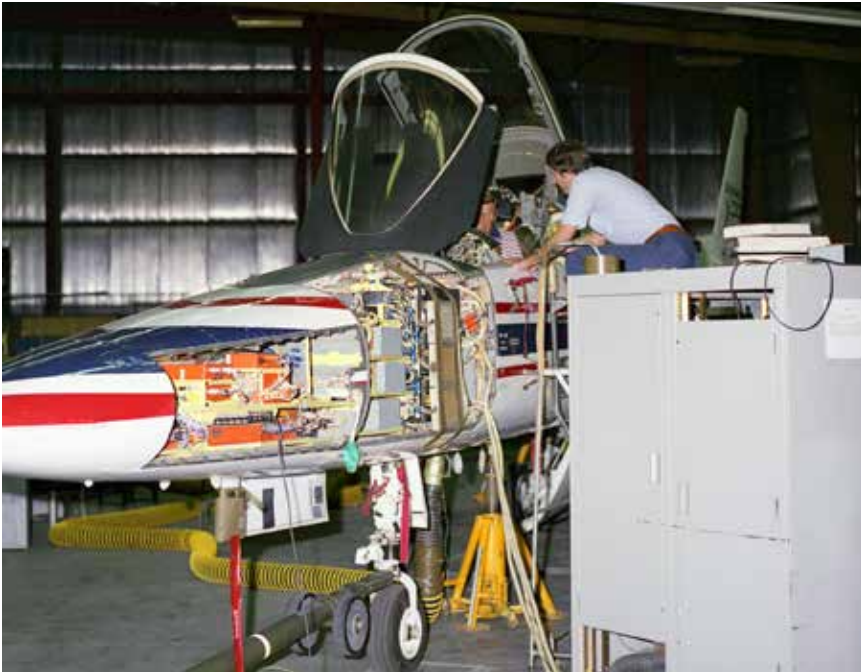
Dryden technicians perform maintenance work on the first Grumman X-29, August 1985. Note flight-test instrumentation racks in forward nose bay. (NASA)
