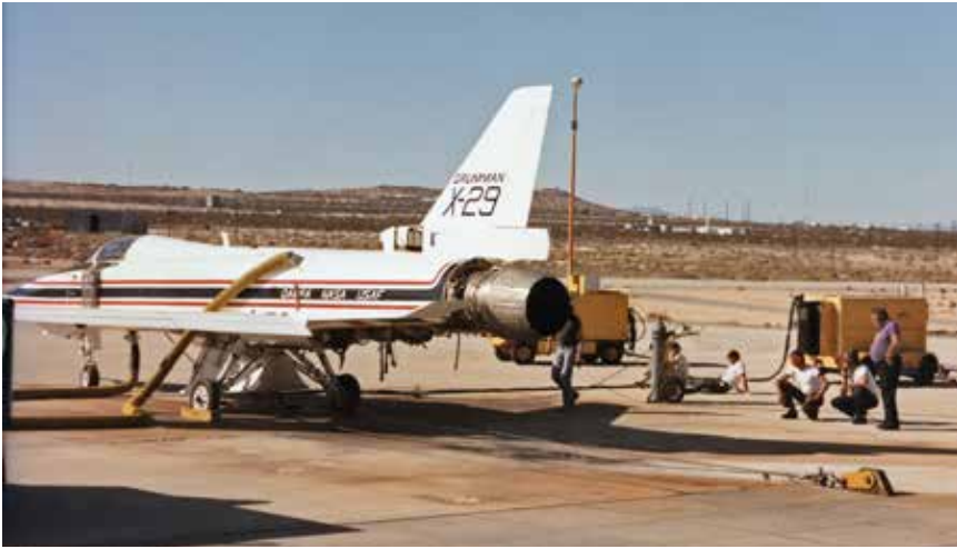
F404 engine test of the first X-29, November 1984, prior to initial flight trials. (USAF via NASA)
