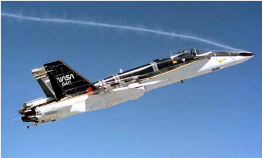
The NASA F/A-18 HARV high-AoA research aircraft during a research flight over the Edwards range. (NASA)
