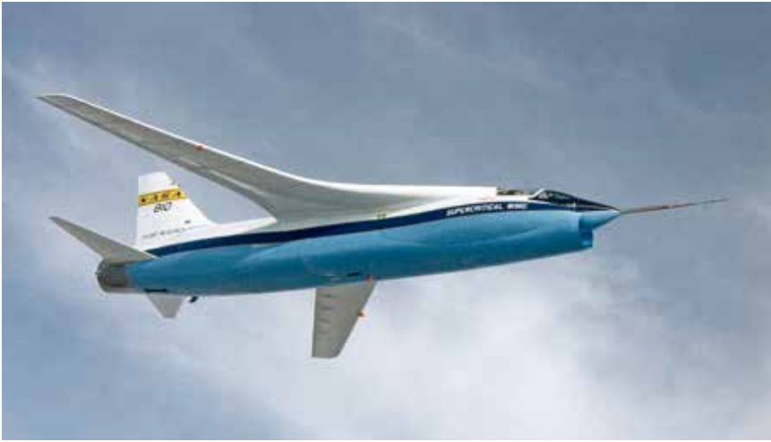
Figure 3.5. Whitcomb's supercritical wing flown on a modified F-8 in 1973.
