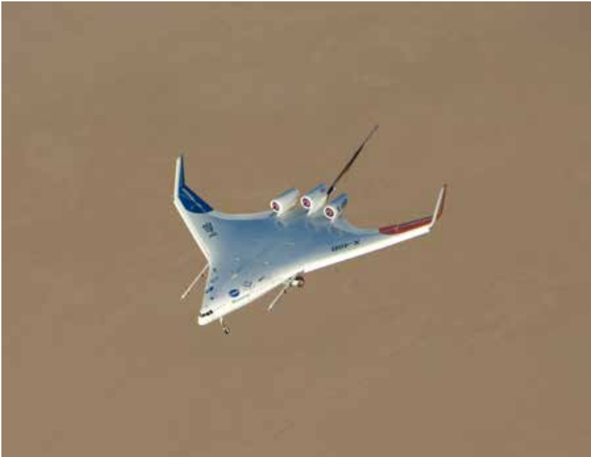
Figure 7.2. X-48B scale model undergoing tests at Dryden in 2007.
