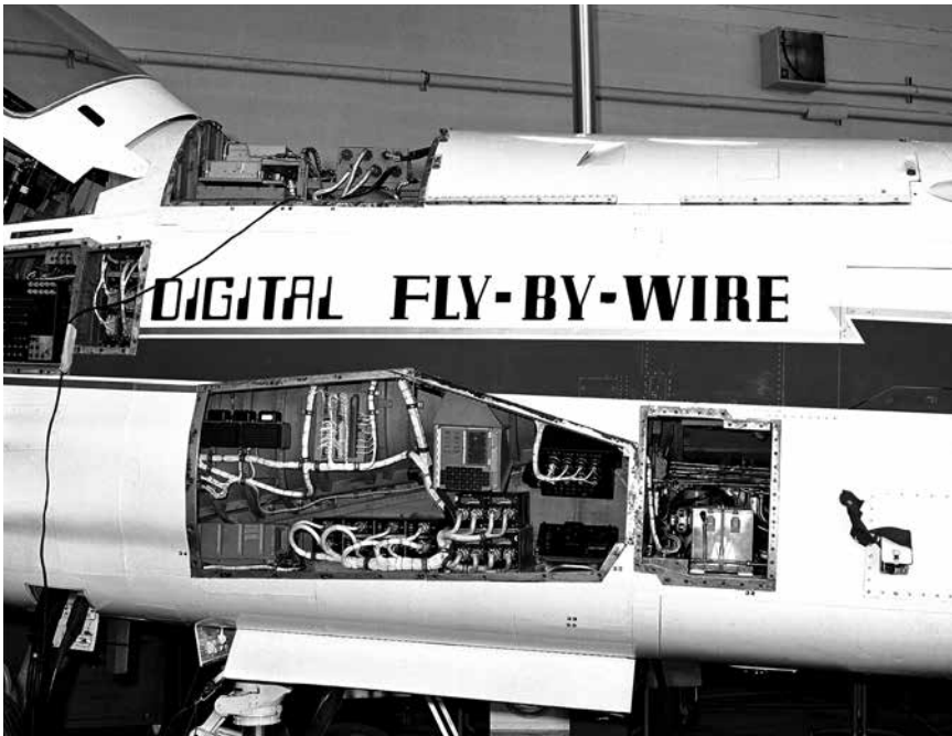
Figure 4.2. Digital fly-by-wire electronics installed in Dryden's F-8 aircraft, 1971.
