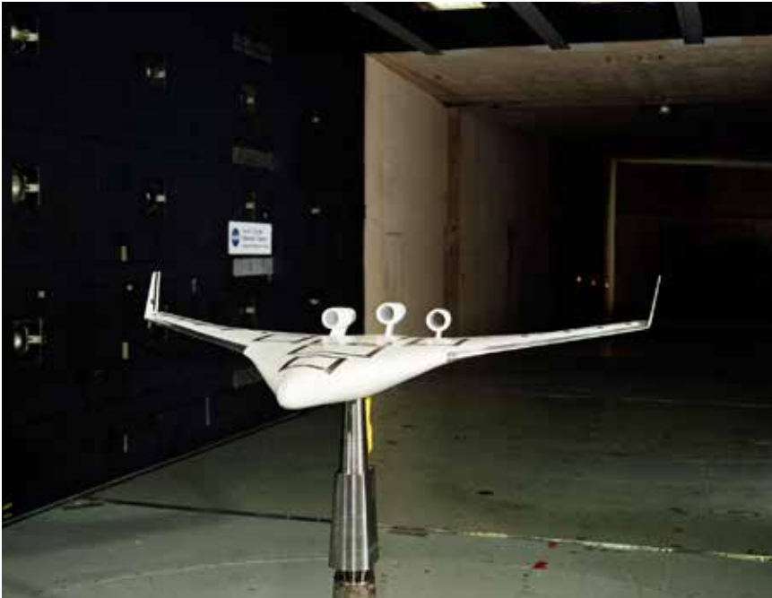
Figure 7.1. Blended wing body model in the Langley 14-by-22-foot wind tunnel.
