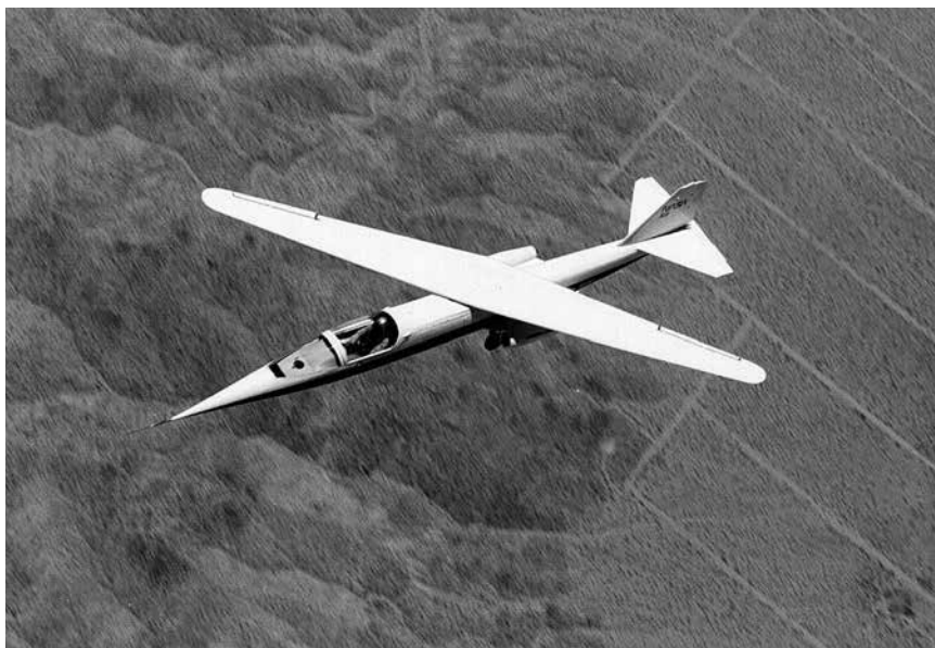
Figure 5.1. AD-1 exhibits its full 60-degree wing sweep in flight.
