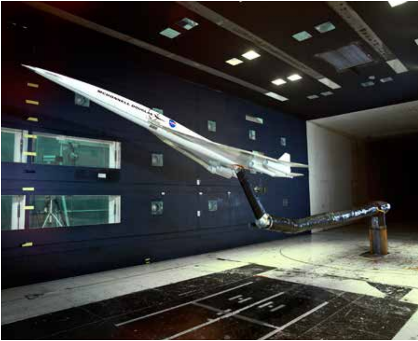
Figure 6.2. High Speed Research model in Langley's 14-by-22-foot tunnel, 1995.
