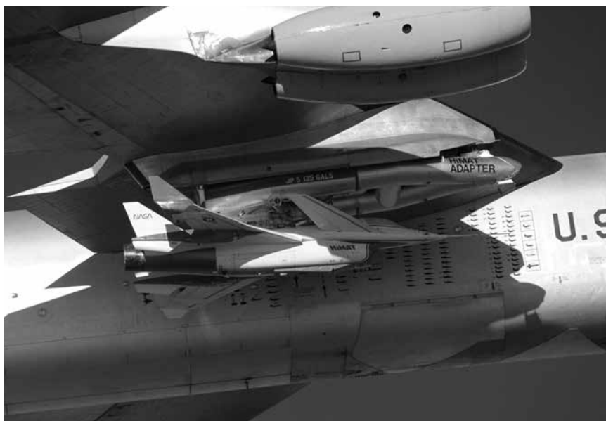
Figure 5.2. The HIMAT remotely piloted vehicle attached to its B-52 mother ship prior to airdrop.
