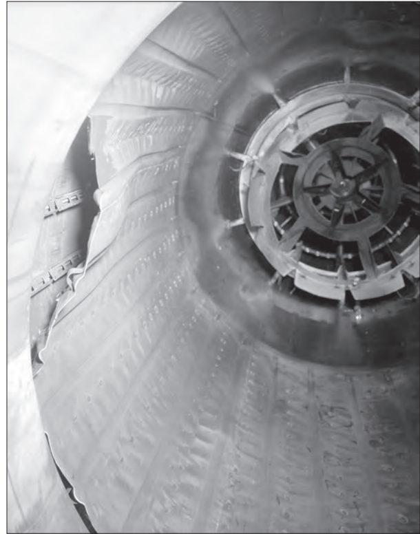
Image 75: Damage to an XRJ47-W-5 combustion liner on 21 March 1955. (NASA C-1955-37979)
