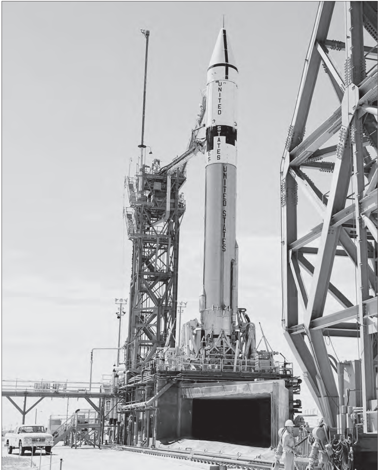
Image 101: Tanking of the Atlas/Centaur-3 rocket at Cape Kennedy on 25 March 1964. The Centaur second stage is behind the white insulation panels near the top. The payload is in the conical nose fairing. (NASA C-1964-68973)
