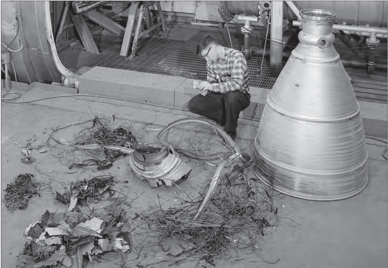
Image 99: John Kobak examines the remains of a failed liquid-hydrogen-cooled engine on 14 June 1960. (NASA C-1960-53702)
