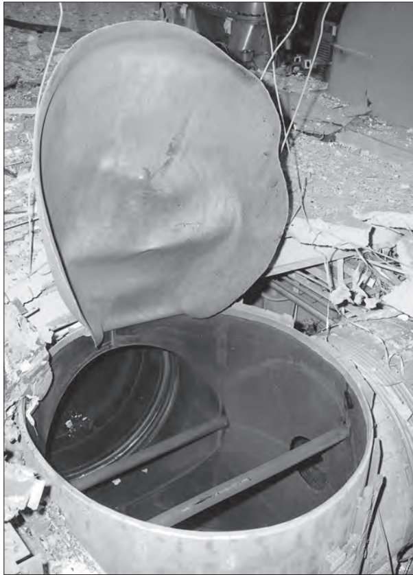
Image 128: Close-up of the 96-inch-diameter header that failed in the explosion. (NASA C-1971-01283)
