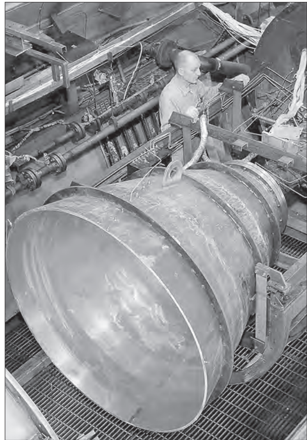
Image 110: An Apollo contour engine is installed in PSL No. 1 on 13 March 1964. Cylindrical and conical combustion chambers were used on the engines. Large-area-ratio nozzles with 15° conical skirts could be used with any of the combustion chambers. Two contour nozzles were machined specifically for a particular chamber. Several injectors were studied, and three were selected for in-depth investigation. (NASA C-1964-68789)
