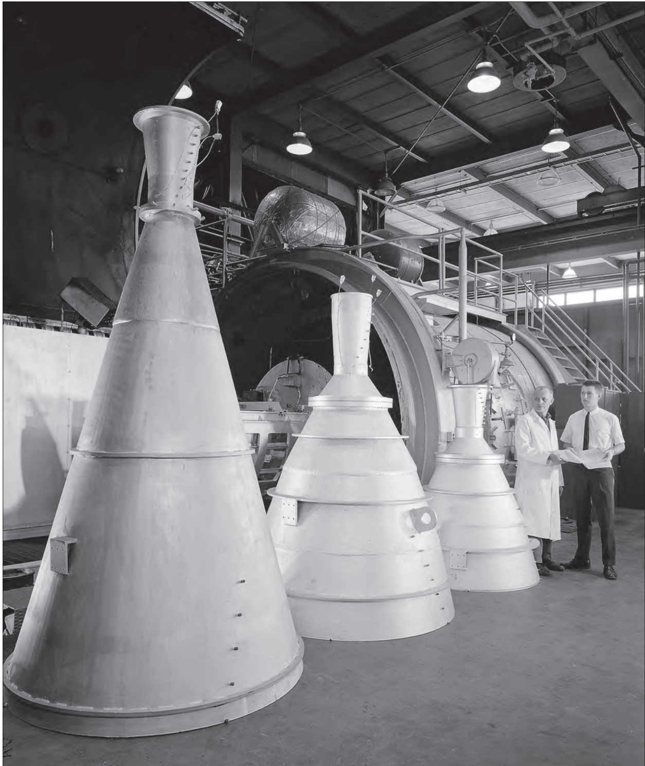
Image 108: Several large-area-ratio nozzles are lined up on 1 May 1964 in front of PSL No. 1 for tests with “storable” propellants. Nozzles (left to right): 15° conical, Apollo Space Propulsion System contour, and U.S. Air Force Titan transtage contour. The veteran mechanic Bill Neidengard is examining the nozzles with a young researcher. (NASA C-1964-69633)
