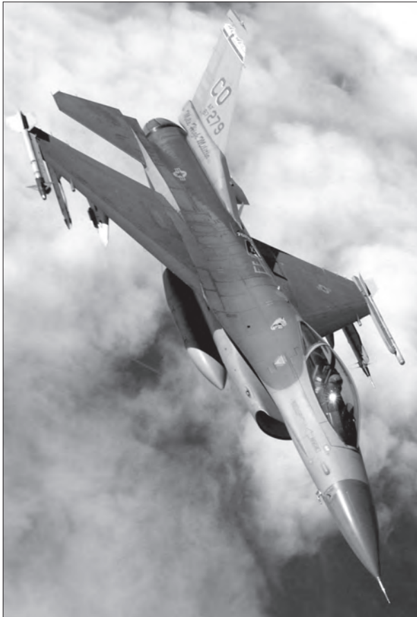
Image 143: The F-16 Falcon was powered by the 27,000-pound-thrust F100-PW-200 turbofan. It flew more sorties than any other aircraft during Operation Desert Storm. 18 (2003, U.S. Air Force)
