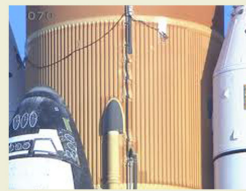
External tank stringer
