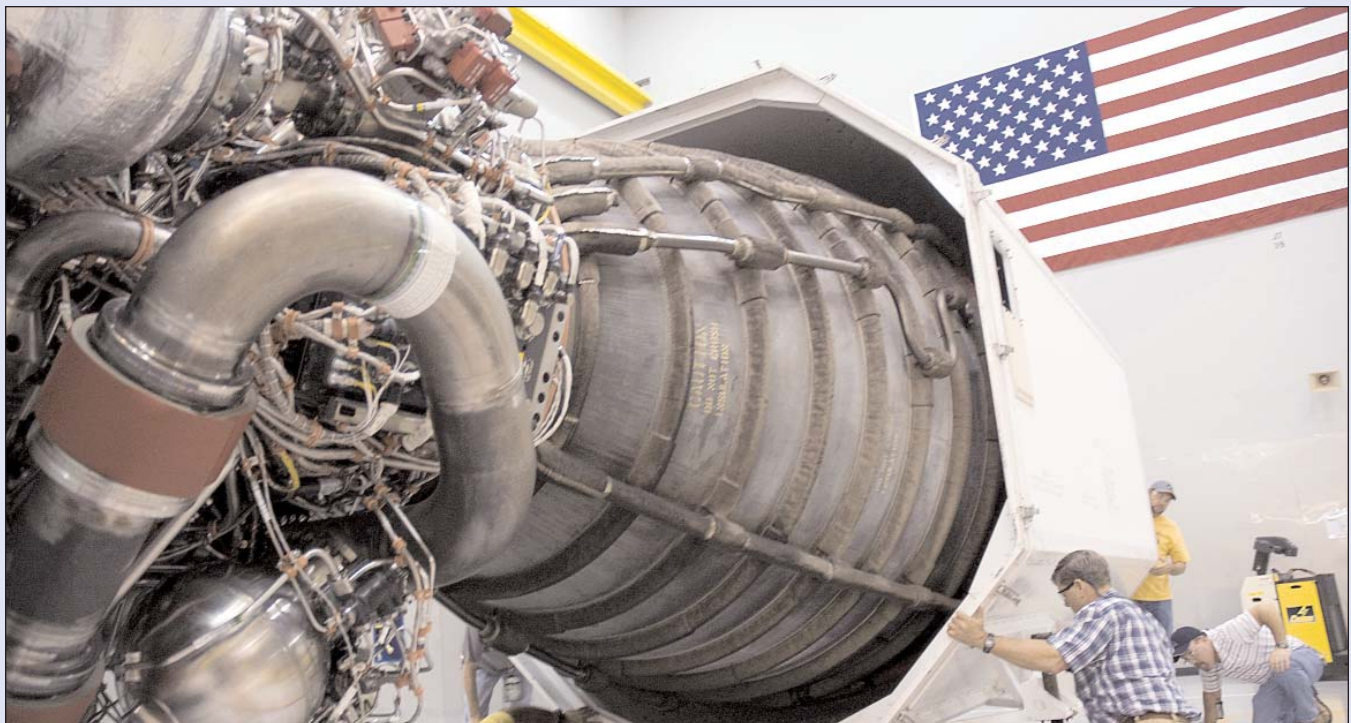
Stennis employees “unpack” space shuttle main engine No. 2061 on Oct. 1, 2008, in preparation for testing it for flight readiness.
