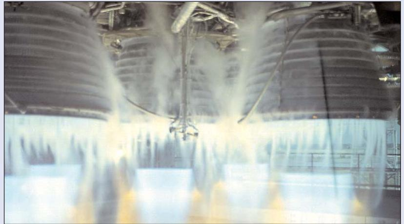
(Right photo) A closeup photo shows the energy blast produced during a test firing of an S-II Saturn rocket engine stage at Stennis Space Center in June 1969
