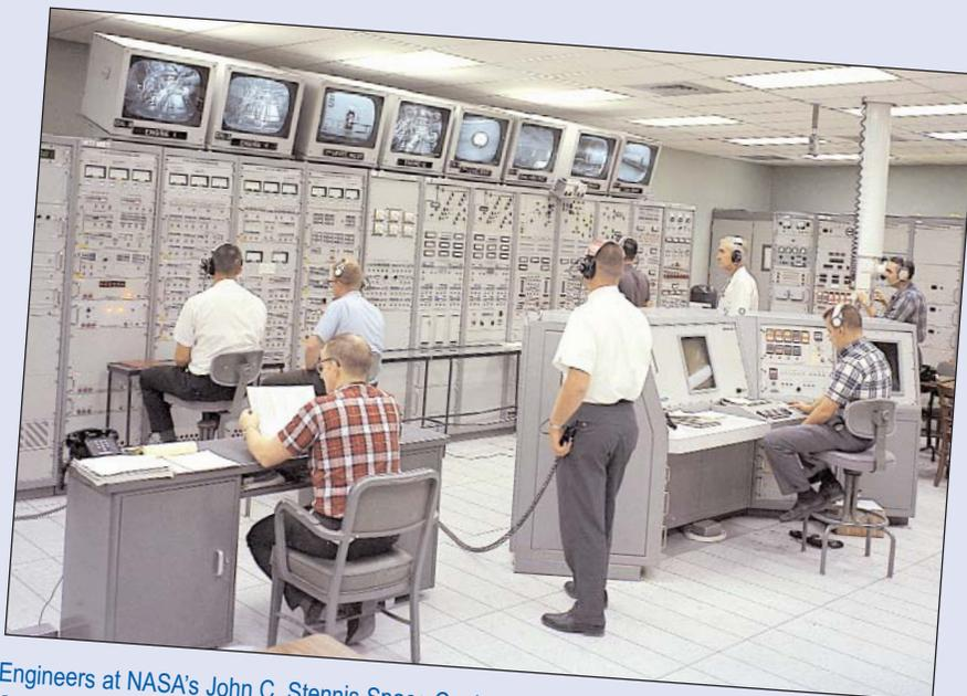
Engineers at NASA's John C. Stennis Space Center monitor a test from the S-II Control Center in October 1966.
