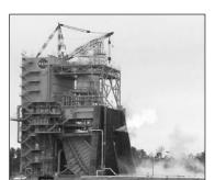
Smoke and flames bear evidence of the success of an April test of the J-2X power pack 1A at the A-1 Test Stand.
