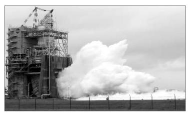
Steam blasts out of the A-2 Test Stand during an Oct. 22 test of space shuttle main engine No. 2061, the last shuttle flight engine scheduled to be built.
