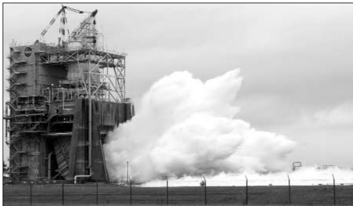
Steam blasts out of the A-2 Test Stand during an Oct. 22 test of space shuttle main engine No. 2061, the last shuttle flight engine scheduled to be built.
