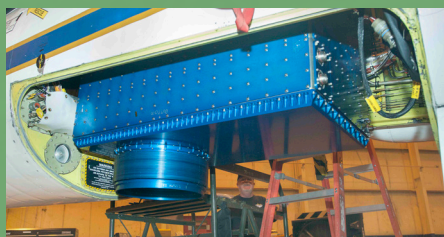
The HSRL-2 instrument is installed into the Q-bay on the ER-2 high-altitude aircraft at NASA's Armstrong Flight Research Center in California.
