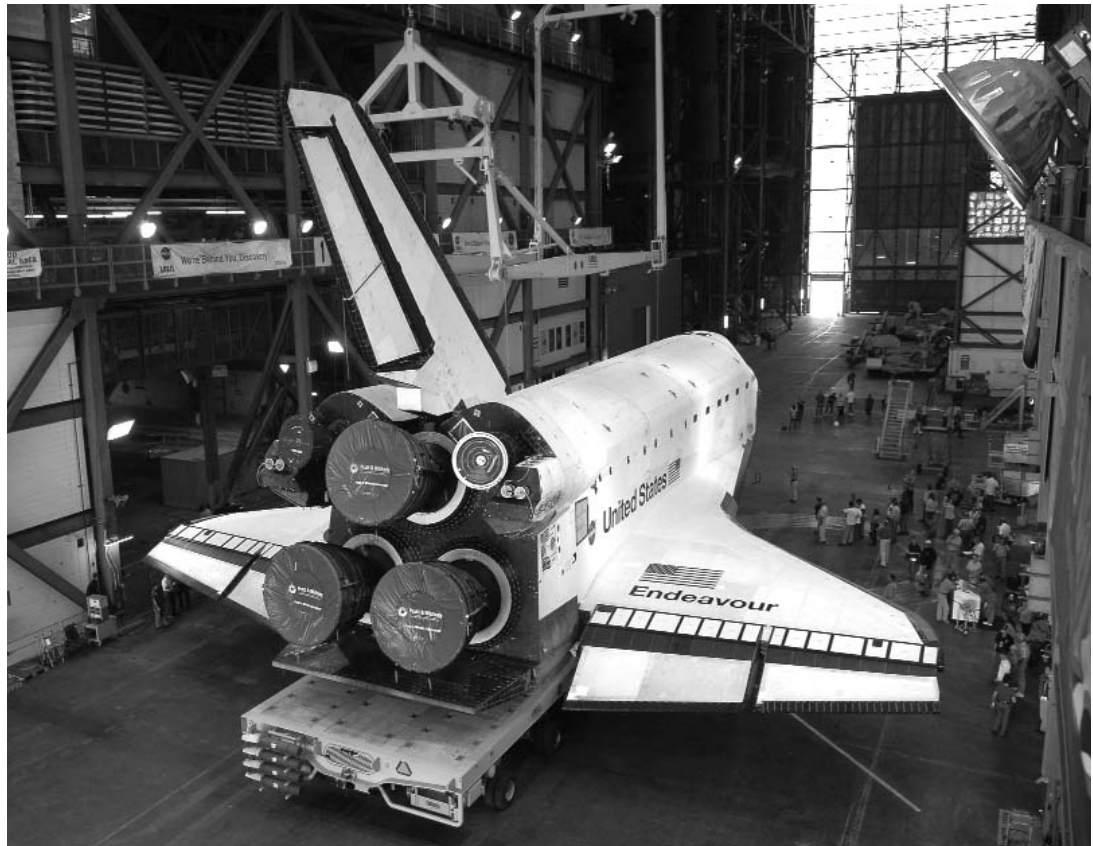
The orbiter Endeavour stops under the overhead crane in the transfer aisle of the Vehicle Assembly Building at Kennedy Space Center, Fla., on July 2. All space shuttle main engines, including the three installed on Endeavour (visible in the photo above), are tested at Stennis Space Center.
