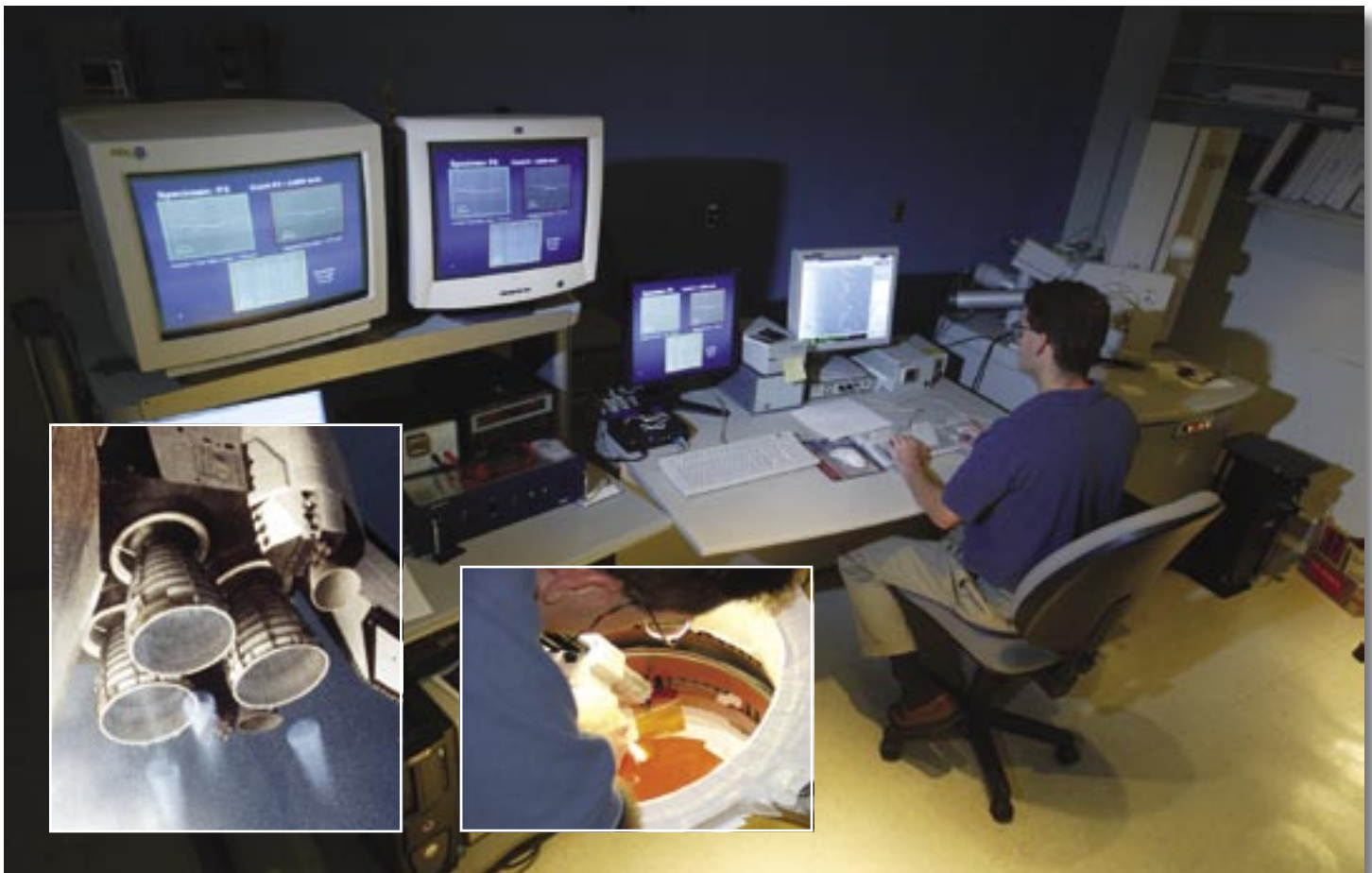
Scott Willard of LaRC identifying cracks in the Space Shuttle Main Engine flowliners. Flowliner slot surface replicas are made (right inset) and then examined under a scanning electron microscope.
