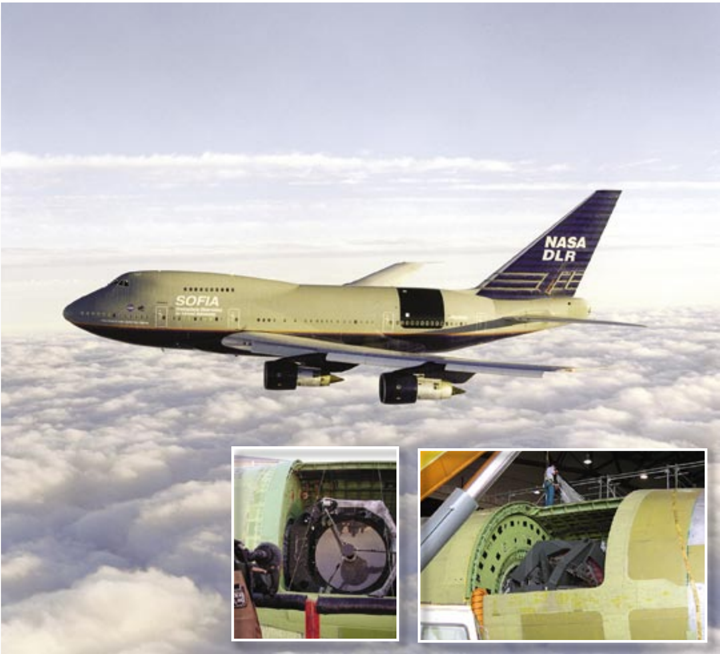
The NESC is focused on the potential for acoustic resonance generated by the infrared telescope cavity in the side of the NASA 747SP aircraft.
