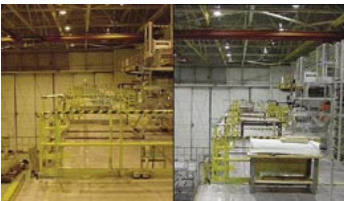
Good lighting is essential for the accurate application of external tank foam and the performance of inspections. Photographs taken before and after NESc involvement.
