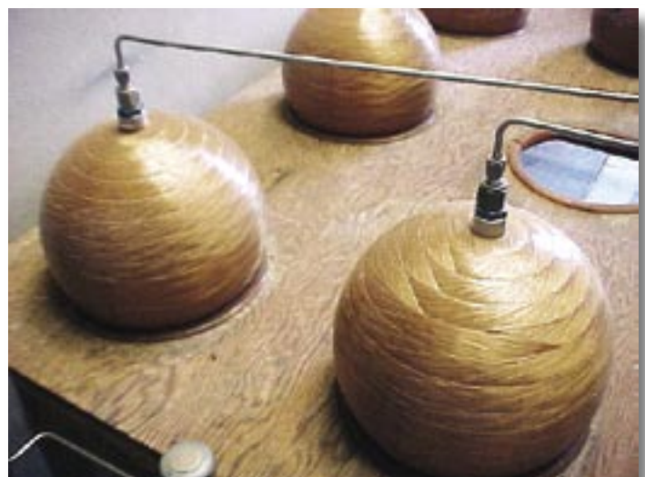
Space Shuttle composite overwrapped pressure vessels being pressure tested.
