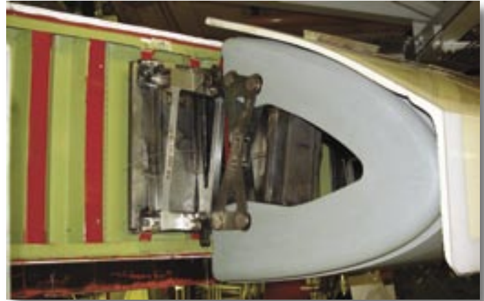
Orbiter RCC wing leading edge (gray) is secured to the wing spar (green) via attachment hardware.
