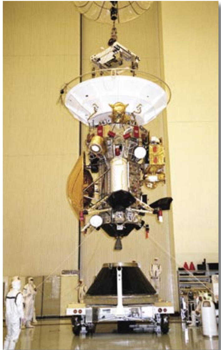
Cassini spacecraft with Huygens probe just visible behind the gold foil covered heat shield.
