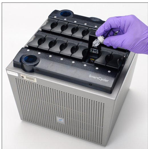
The Wetlab-2 system includes a Cepheid SmartCycler instrument that can perform up to 16 PCR reactions in parallel. Image credit: NASA / Dominic Hart
