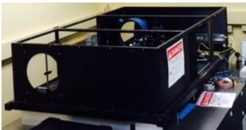
LTES used for generating 20 cm diameter collimated beacon
