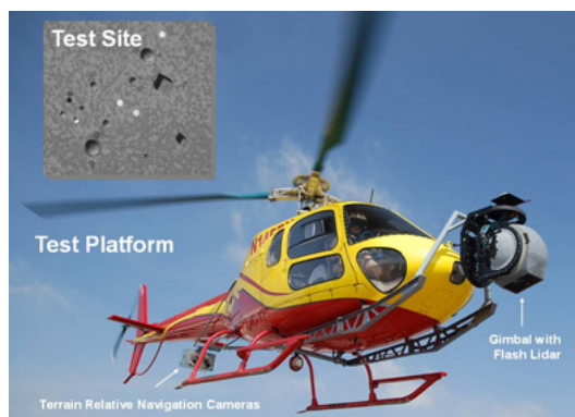
Figure 13. The ALHAT project seeks to develop planetary landers that can automatically recognize a landing site, assess potential landing hazards, and adjust accordingly during descent.
