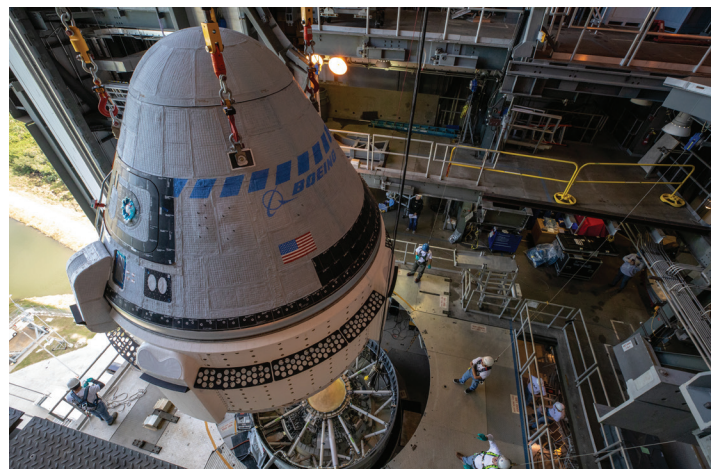
Below: Risk analysis is reviewed for launches. Here the Boeing CST-100 Starliner is guided into position above a United Launch Alliance Atlas V rocket at the Vertical Integration Facility at Space Launch Complex 41 in November 2019.
