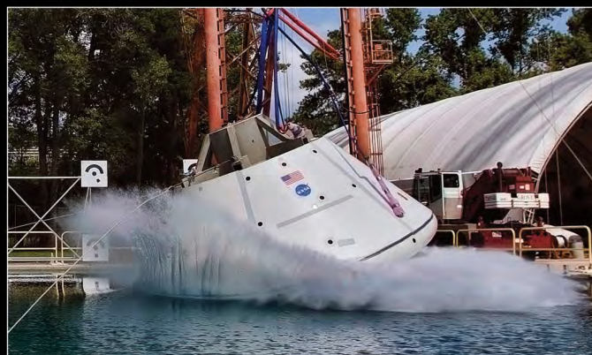
An 18,000-pound test version of Orion, which was built and designed at Langley, was dropped into Langley's Hydro Impact Basin, simulating what the spacecraft may encounter when landing in the Pacific Ocean.
