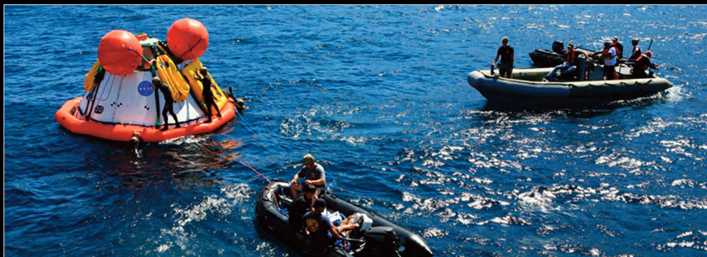
An Orion mockup, built and designed at Langley, floats in the Pacific Ocean during an Underway Recovery Test.
