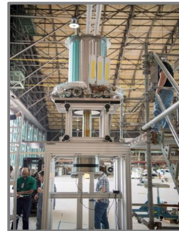
KRUSTY Assembly with Simulated Reactor Core on Comet Mock-up in GRC Hangar – September 2017
