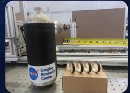
Demonstrate winding a 4" diameter pressure vessel
