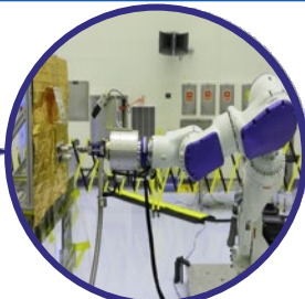
Remote Robotic Oxidizer Transfer Test 2014
