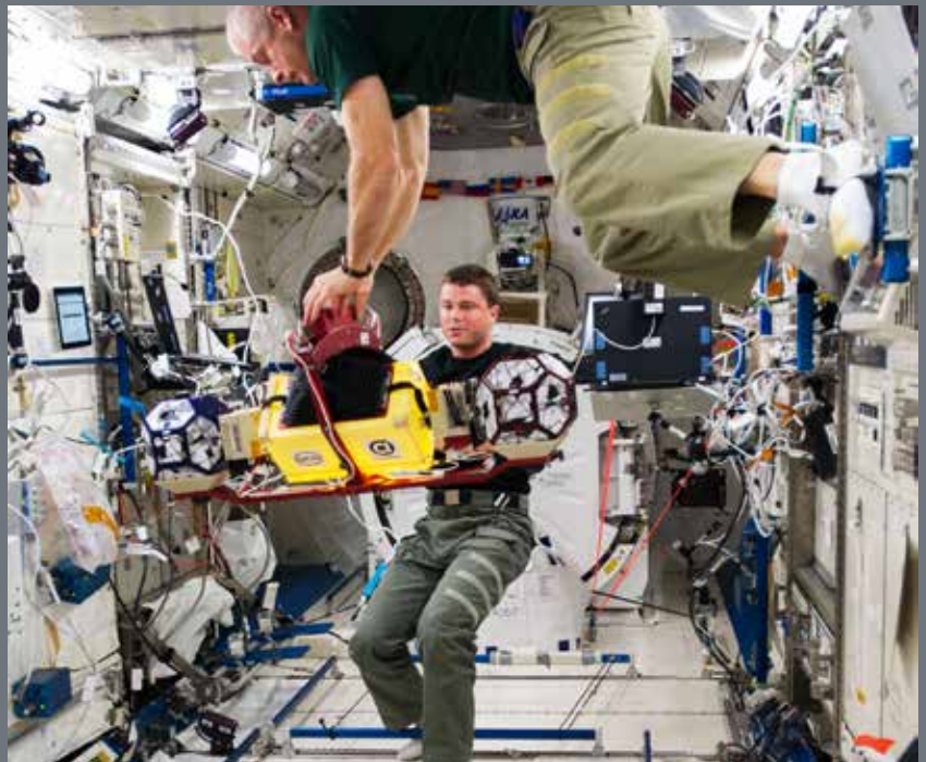
In the International Space Station's Kibo laboratory on June 18, 2014, NASA astronauts Steve Swanson (top) and Reid Wiseman, conduct test runs of the SPHERES-Slosh experiment, using the soccer ball-sized, free-flying satellites known as Synchronized Position Hold, Engage, Reorient, Experimental Satellites, or SPHERES. The SPHERES-Slosh investigation uses small robotic satellites on the space station to examine how liquids move around inside containers in microgravity.
