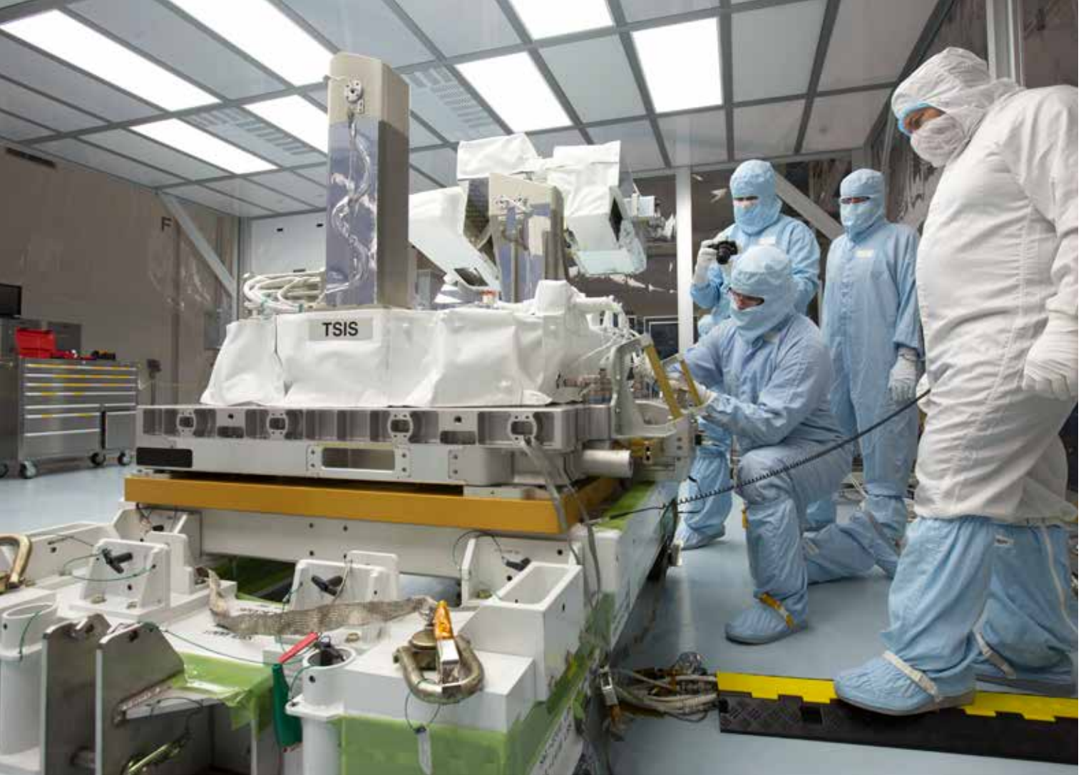
In the high bay of Kennedy's Space Station Processing Facility, Chris Hardcastle, left, of Stinger-Ghaffarian Technologies, performs a sharp-edge inspection of the integrated Total and Spectral Solar Irradiance Sensor-1 (TSIS-1) payload and the EXPRESS Pallet Adapter. Hardcastle is joined by Dwayne Swieter, right, a TSIS-1 payload team member from the Laboratory for Atmospheric and Space Physics, a Research Institute at the University of Colorado (Boulder). Designed to measure the Sun's energy input into Earth, TSIS-1 launched on SpaceX's 13th commercial resupply mission to the International Space Station.
