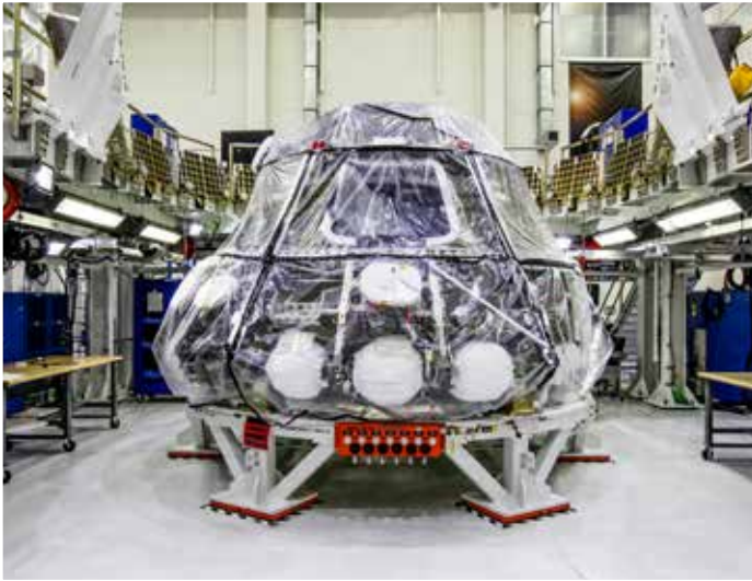
The Orion crew module for NASA's Exploration Mission-1 (EM-1) is secured in a work station May 11, 2017, in the Neil Armstrong Operations and Checkout Building high bay at NASA's Kennedy Space Center. Orion will undergo additional processing to prepare it for launch on its first integrated flight atop the Space Launch System rocket on EM-1.
