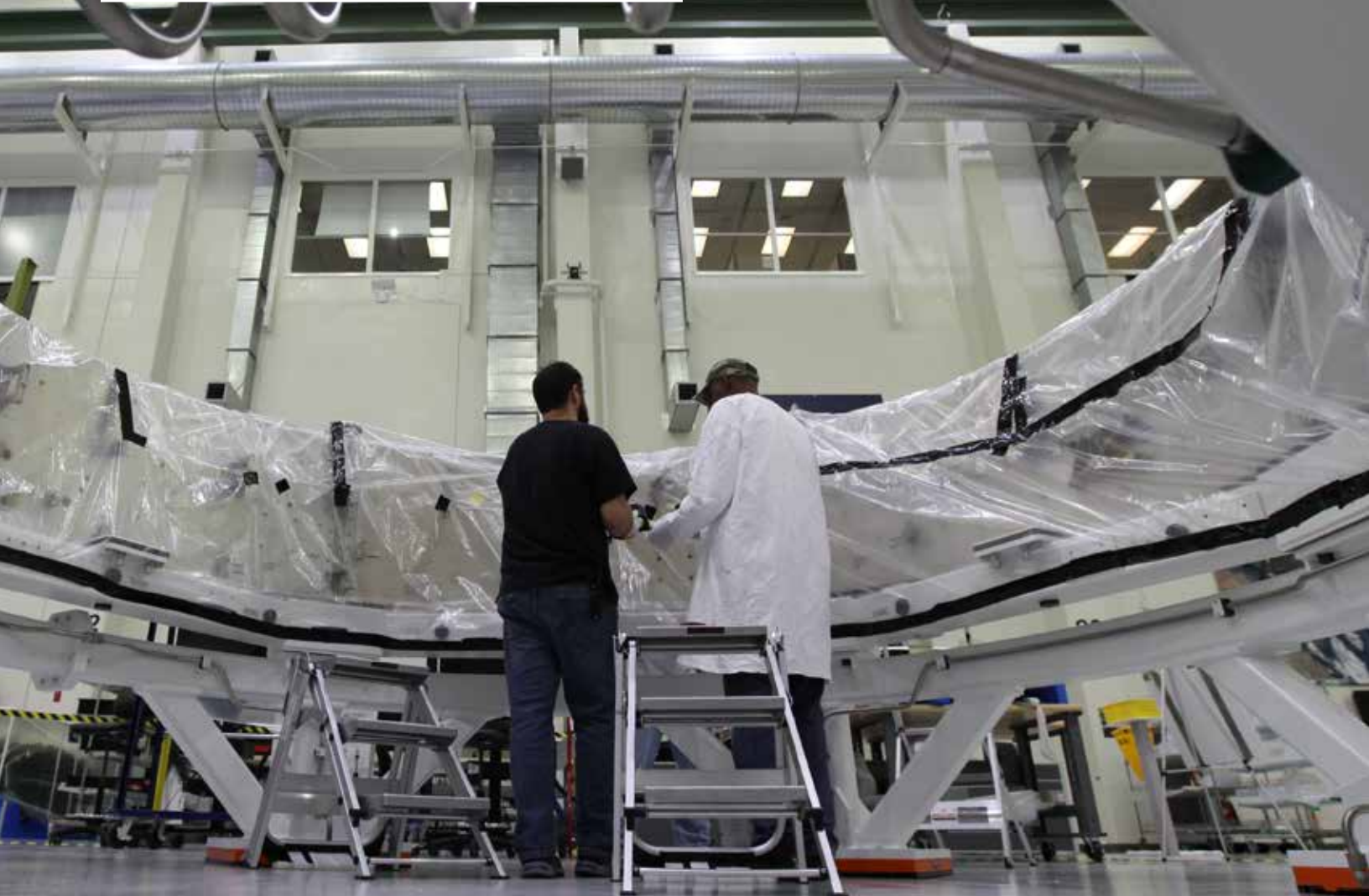
Inside the Neil Armstrong Operations and Checkout Building high bay at NASA's Kennedy Space Center, Lockheed Martin technicians secure a protective cover around the Orion crew module adapter (CMA) for Exploration Mission-1. The CMA was moved to a clean room to undergo propellant and environmental control and life support system tube installation and welding. The adapter will connect the Orion crew module to the European Space Agency-provided service module.
