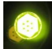
7-hole W-UO 2 in CFEET and post testing up to 2500 C
