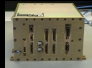
Controller Electronics (CE) Engineering Development Unit (EDU)
