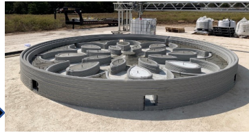
The 3D printed subscale prototype of the Lunar PAD ready for hot fire testing at Camp Swift. Photo via ICON.
