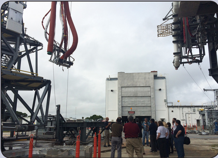
Members of the media tour the Launch Equipment Test Facility on Dec. 1 at NASA's Kennedy Space Center in Florida. Above them is the Orion Service Module Umbilical being prepared for testing on Vehicle Motion Simulator 1. Photo credit: NASA/Amber Philman
